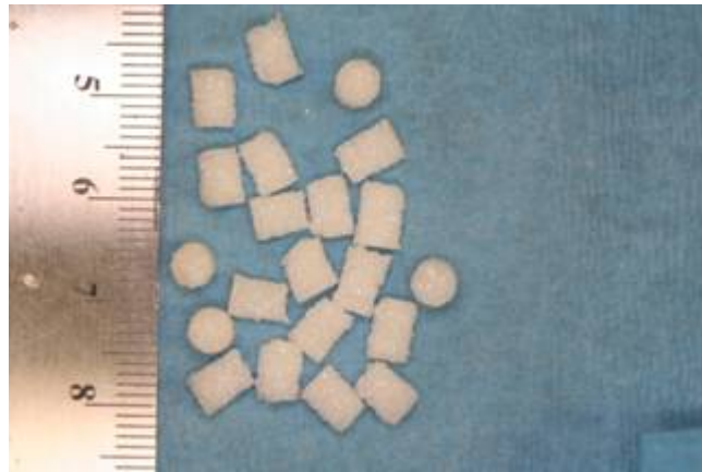
Figure 4.2.1a: Picture of PLGA scaffolds showing similar size and shape
