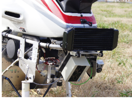
Figure 8: A LIDAR (Sick LD-MRS HD) fitted to the Georgia Tech UAV test-bed to scan vertically.
