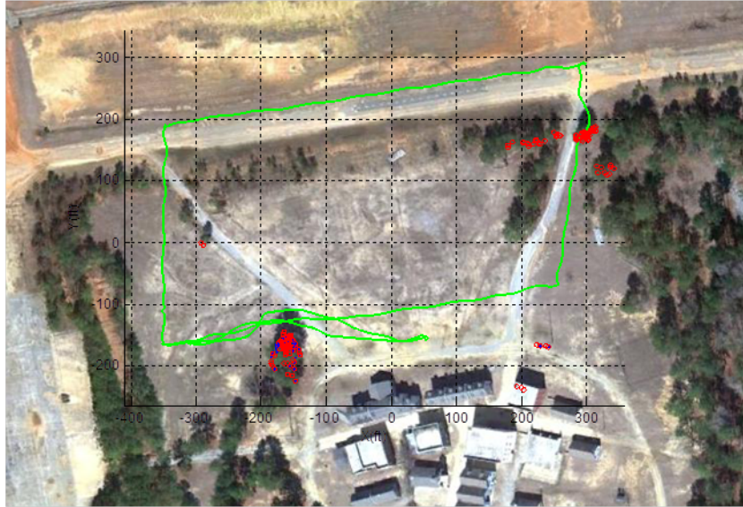
Figure 85: McKenna MOUT site flight test trajectory ( 15\text{ft/s} ): Top projection.
