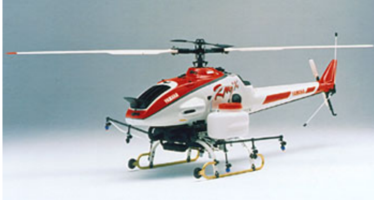
Figure 96: Original Yamaha RMAX is designed for agricultural and industrial use.
