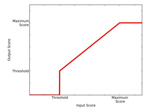
Figure 13: The Threshold Transformation Function
