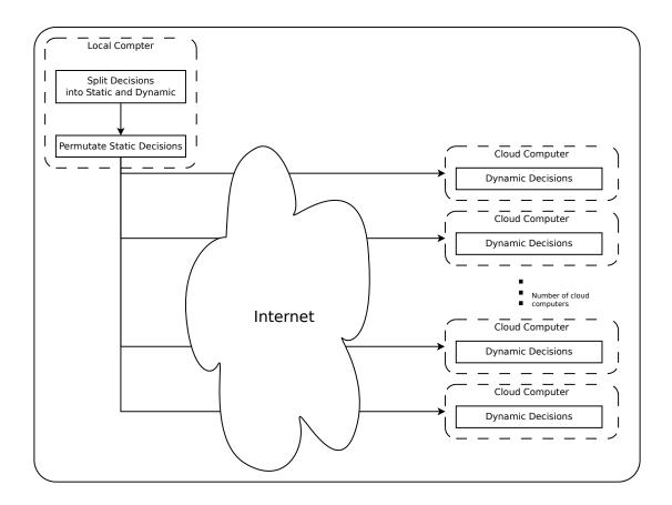
Figure 28: Architecture of RAAM on the Cloud
