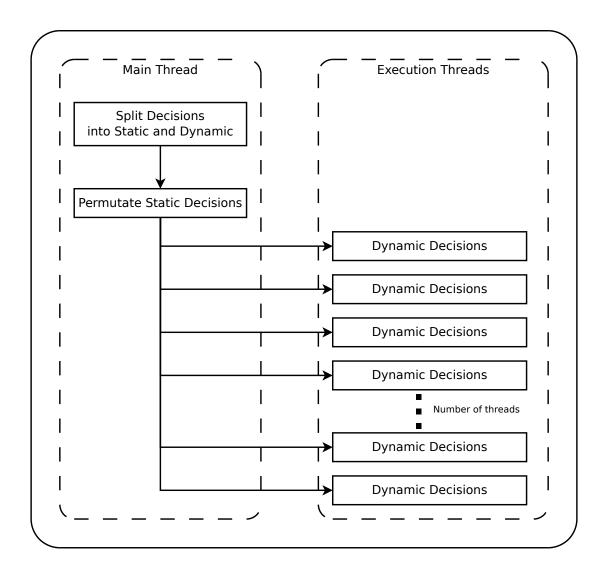
Figure 27: Decision Allocation between Threads
