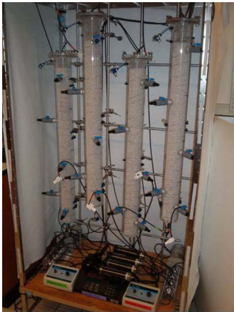
Figure A-1 Reactors prior to startup, showing initial color of pumice, locations of sample ports, and media and lactate pumps.
