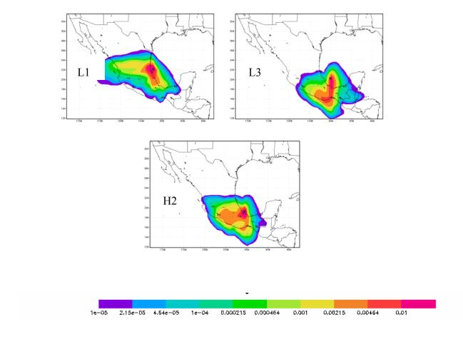
Figure 49. Influence regions (normalized) for measurement locations over the gulf where the combustion CO:CO<sub>2</sub> ratio was low (L1 and L3) and where the combustion CO:CO<sub>2</sub> ratio was high (H2). The warm colors indicate regions of strong influence and the cool colors indicate regions of less influence.
