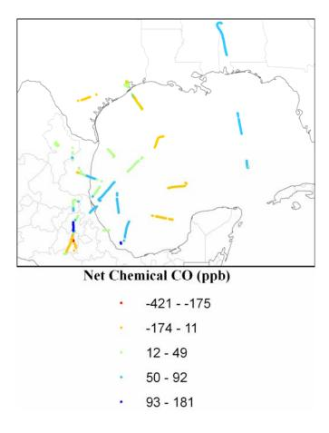
Figure 47. The net chemical contribution to the modeled CO component along the flight paths. Flight paths are limited to those having observed CO<sub>2</sub> mixing ratios above 385 ppm.
