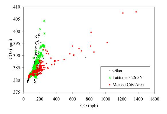
Figure 41. Observed mixing ratios of CO vs. CO<sub>2</sub> along the INTEX-B DC8 flight paths with observations within 200 km of Mexico City in red, observations above 26.5 degrees north in green (over U.S. and northern Gulf of Mexico), and all other observations in black.
