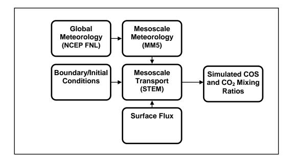
Figure 2. Process diagram for atmospheric transport model.
