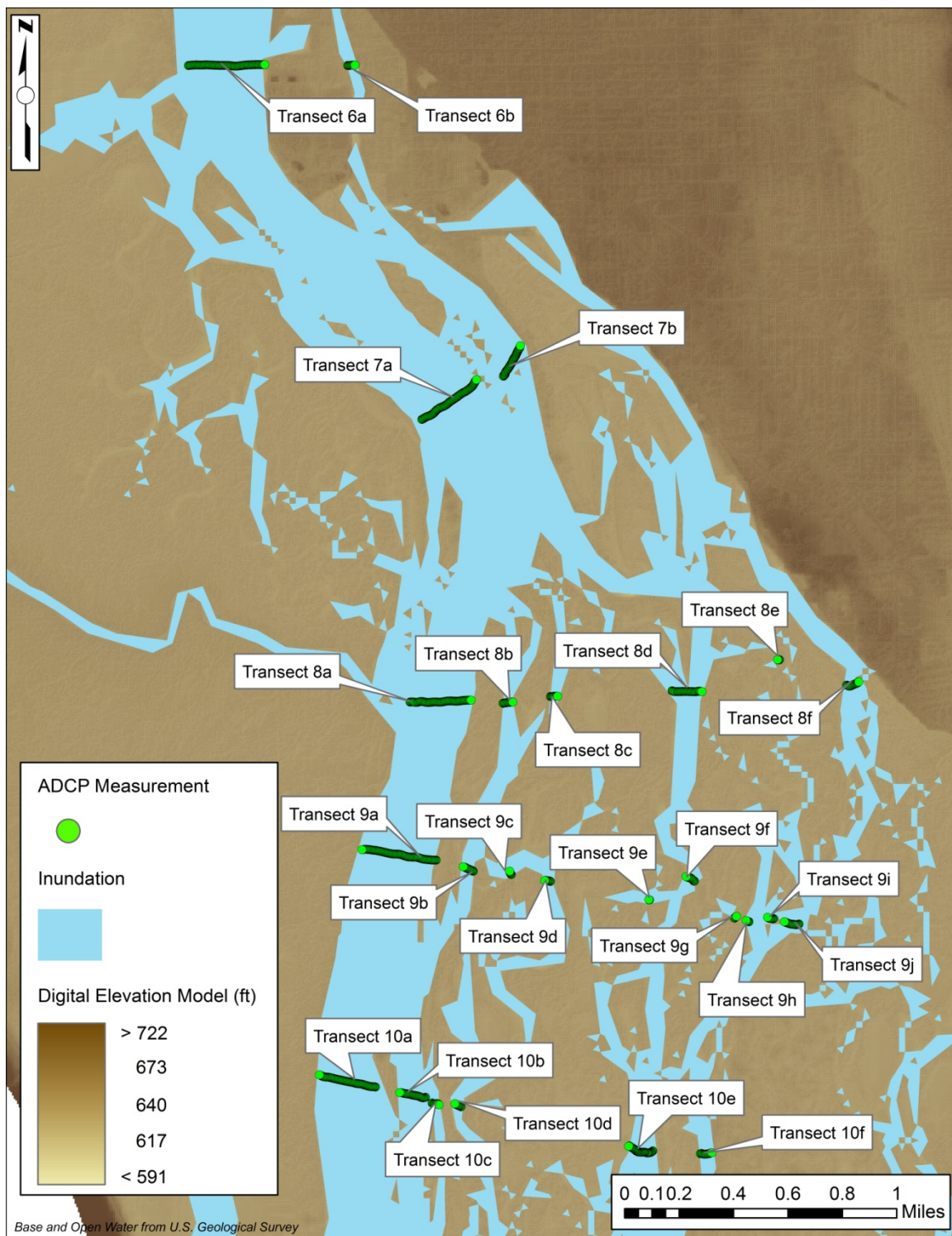
Figure 3.13. ADCP transects 6 through 10 showing location of sub transects (Data Source: USGS, 2010b). Data flooded by dark brown extends to elevation 1,178 feet and data flooded by light brown extends to elevation 561 feet.
