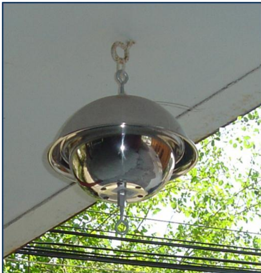
Figure 1-3: Passive sampling device in outdoor environment
