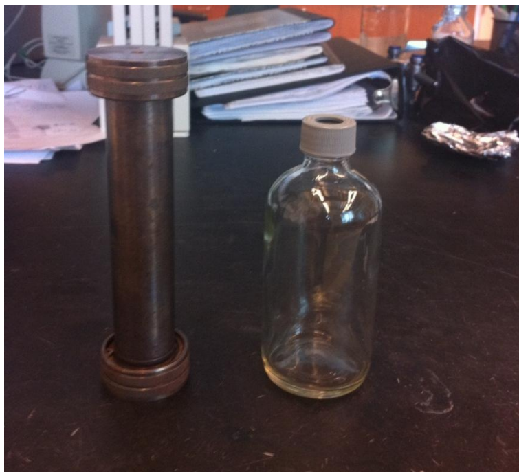
Figure 2-2: ASE Cell (left) and Collection Jar (right)
