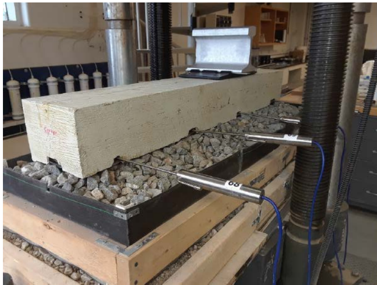
Figure 5.1 Simulated Trackbed for Distribution Testing
