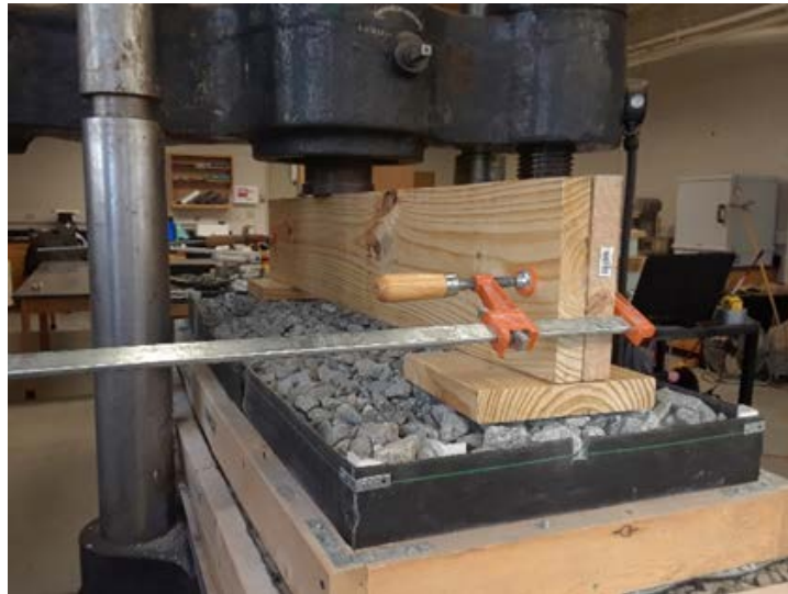
Figure 5.6 Ballast Bed Compaction Attempt
