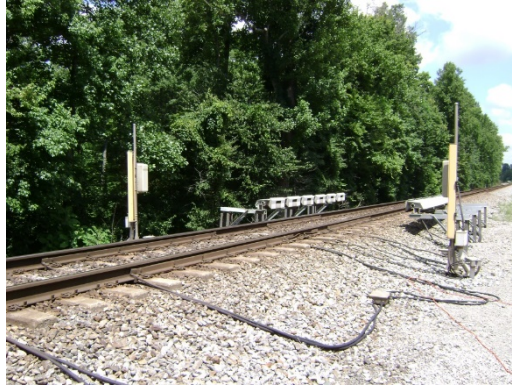
Figure 7.2 Typical Salient Mk-III WILD Installation
