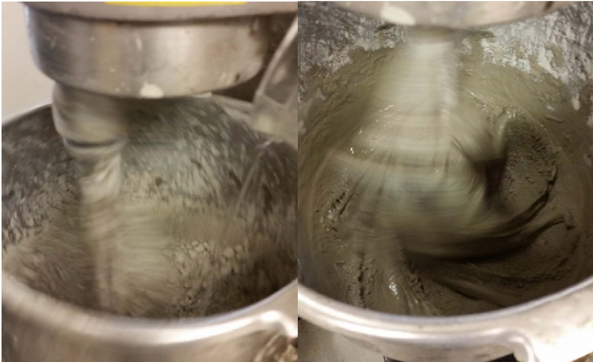
Figure 3.2: Mixing of ingredients in bowl at beginning (left) and end (right) of mixing process.
