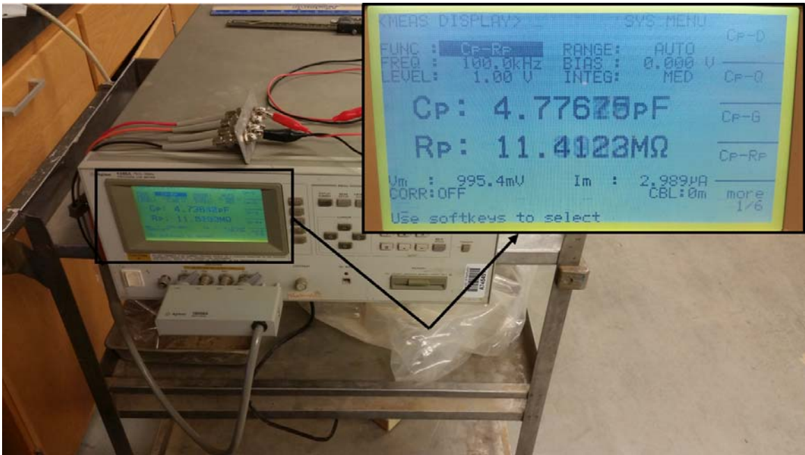
Figure 3.13: Agilent® LCR Meter Model 4285A and attached Agilent® Test Leads Model 16048A. Display screen and settings also pictured.
