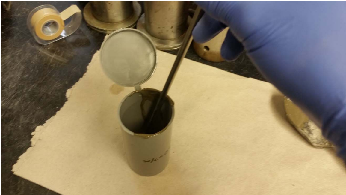
Figure 3.3: Smooth metal rod is used to tamp the mixture after a lift has been poured.
