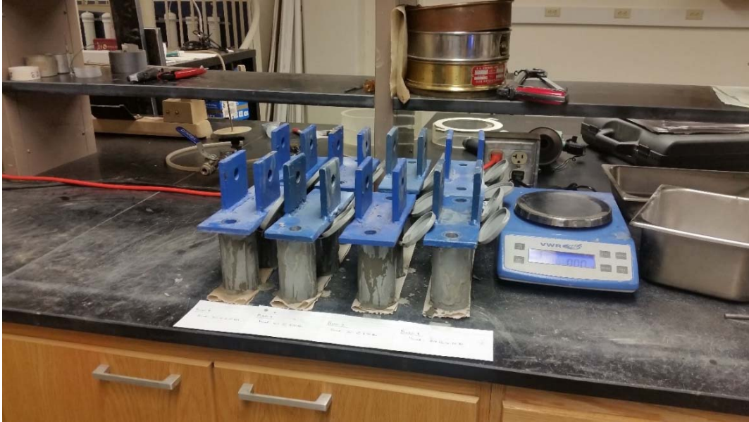
Figure 3.5: 2 kg weights placed on top sample molds during 24 hour hardening phase.
