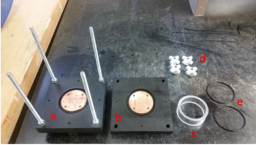
Figure 3.11: Unassembled resistivity cell used to measure electrical properties of DI-water and defoamer mixture. Parts pictured include: (a) bottom plate, (b) top plate, (c) acrylic cylinder, (d) sprockets, and (e) O-rings.
