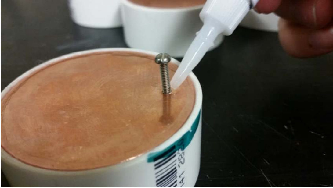
Figure 3.18: Electrode glued to top of PVC mold. Glue was also placed around screw on outside face of electrode.
