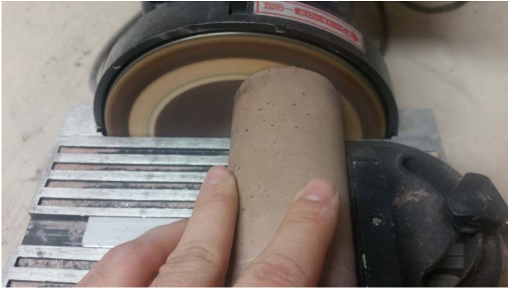
Figure 3.14: Concrete cylinder top surface sanded smooth by the disc sander.
