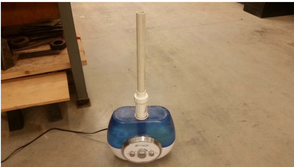
Figure 3.7: Telescoping and straight PVC pieces connected to humidifier.
