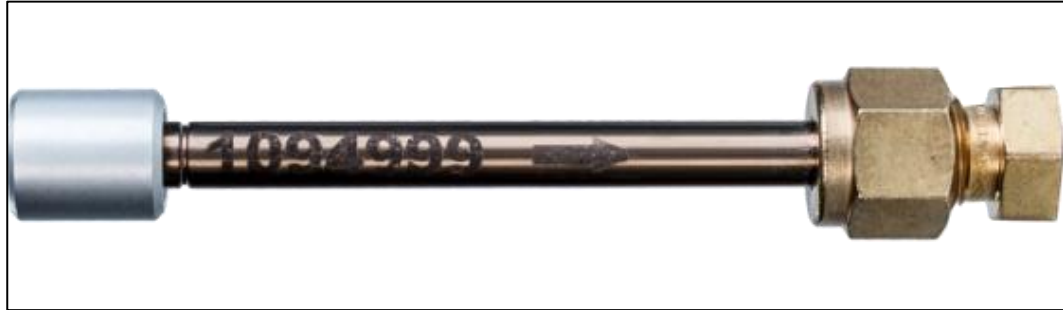
Figure 3-7: Passive sampler with diffusion cap attached
