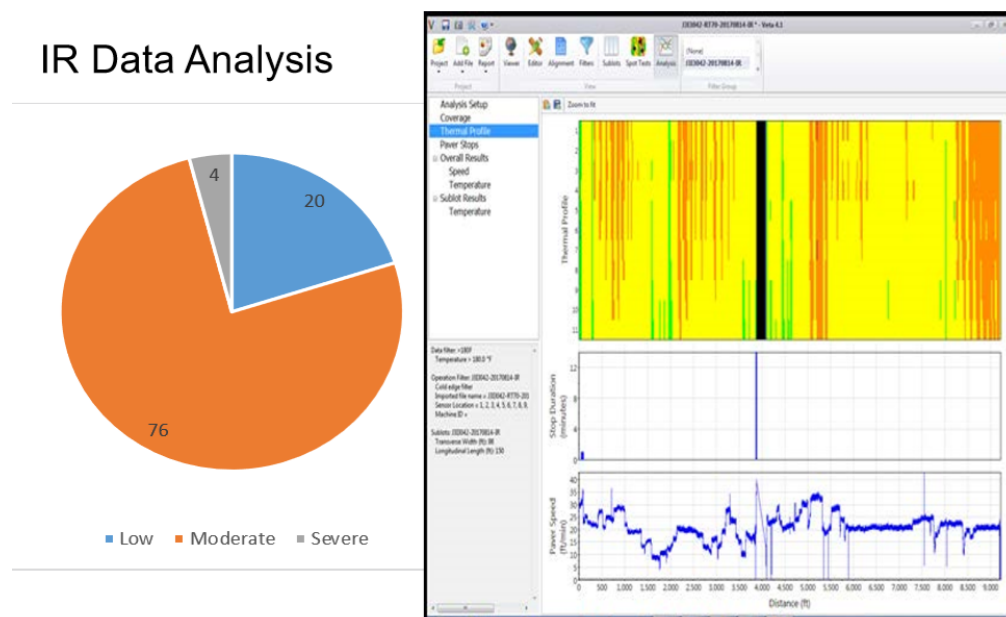
Figure 6.1: Thermal Profile of Mat (FHWA 2018)
