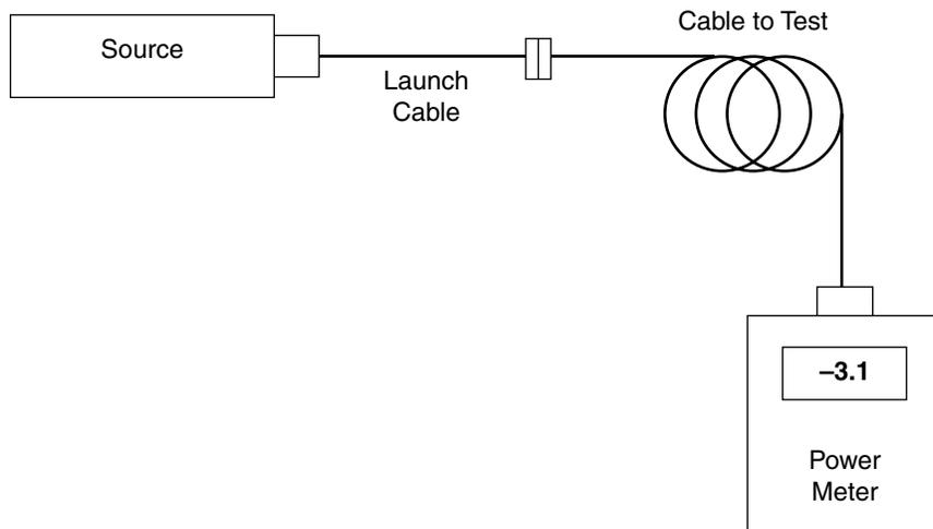
**Figure 17-15** Basic fiber optic cable loss test.
