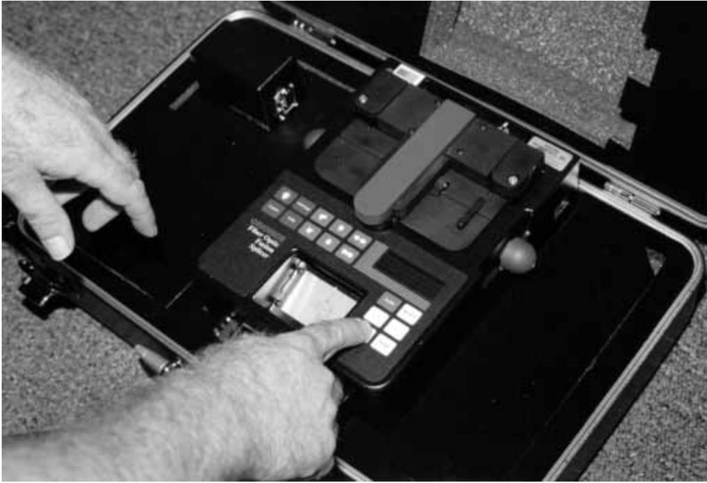
**Figure 6-9** Fusion splicer.
