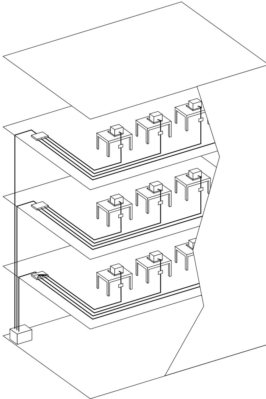
**Figure 7-2** “Homerun” or centralized fiber cabling system.
