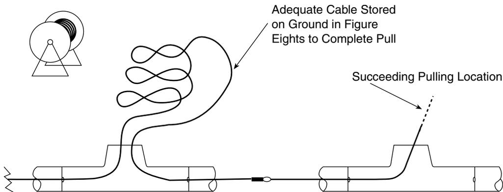
**Figure 15-4** The second half of a multistage pull.
