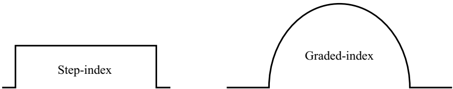
Fig. 1.6. Index profiles representing main multimode fiber designs. Horizontal scale represents radial position in fiber. Vertical scale represents refractive index
