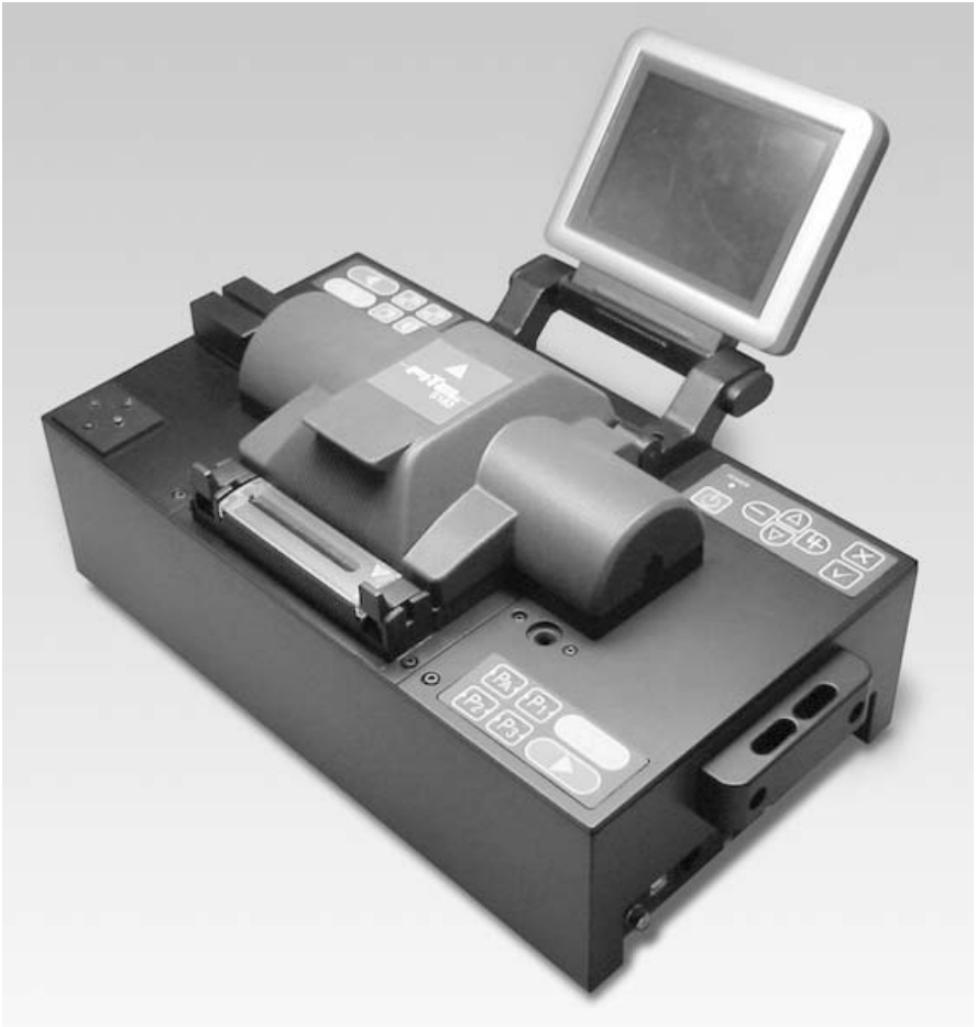
Fig. 10.6. The Fitel S183 is a contemporary arc fusion splicer designed to incorporate a great deal of flexibility so that it can be applied to specialty fibers such as PM fiber in a factory setting as well as in a laboratory environment. The splice cover is in the down position obscuring the view of the fiber chucks and electrodes. A small heater for curing heat shrink splice protectors is visible on the front of the unit opposite the LCD screen mounted on the back. This machine includes a profile alignment system (PAS). Photo courtesy of Furukawa America, Inc.
