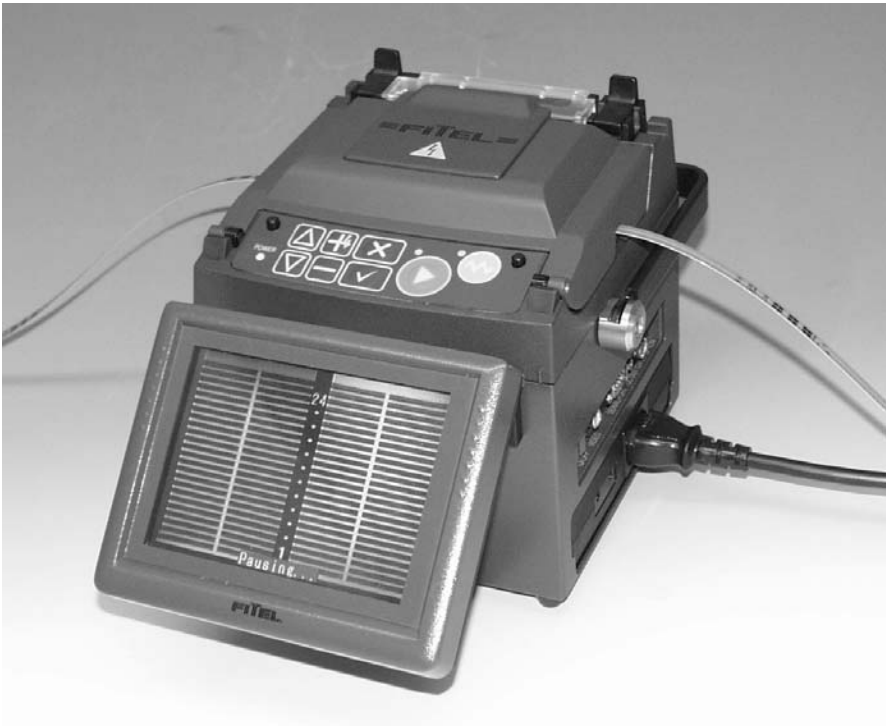
Fig. 10.4. The Fitel S199M24 mass fusion splicer can simultaneously fusion splice all the strands of a 24 fiber ribbon cable. The LCD display on the front of the unit shows two orthogonal views of the 24 individual fiber strands with a small gap between the opposing fiber tips. Typical fusion splice losses are about 0.03 dB for standard single-mode fiber (SMF) and about 0.1 dB for non-zero dispersion-shifted fiber (NZ-DSF). This machine can be used in a field or factory environment. Photo courtesy of Furukawa America, Inc.
