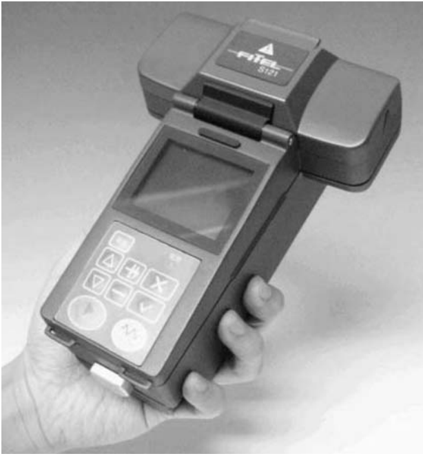
Fig. 10.2. The Fitel S321A is a mini handheld field fusion splicer designed to splice single strands of SMF or MMF. This compact arc-fusion splicer weighs only 1 kg and incorporates battery power, a CCD based alignment system, an LCD monitor, automatic fiber alignment and splicing, a proof-tester, and can even include an oven for curing heat-shrink splice protectors. The time require for alignment and splicing is only about 15 seconds and the splice loss averages about 0.1 dB for SMF and 0.05 dB for MMF. Photo courtesy of Furukawa America, Inc.
