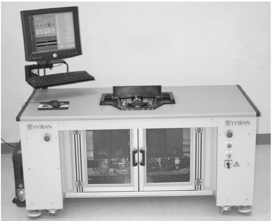
Fig. 10.7. The Vytran FAS represents the automated future of factory fusion splicing since it is a fully automated fusion splicing workstation that can automatically strip, clean, cleave, fusion splice, proof test, package, and estimate splice loss. Fibers are laid up in a pallet arrangement by an operator and this pallet is then automatically processed by the machine. Only about 150 seconds are required to execute all the steps of the fusion splice process. This machine is also notable because it employs a tungsten filament (Fig. 10.10) as a heat source instead of the usual electric arc. Photo courtesy of Vytran Corporation
