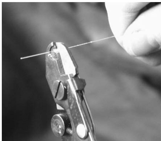
Fig. 2.3. Common optical fiber mechanical stripping tool applied to standard single-mode fiber with a standard 250 \mu\text{m} diameter dual layer acrylate coating
