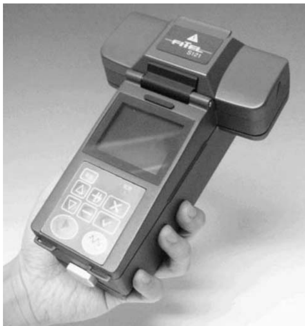
Fig. 10.2. The Fitel S321A is a mini handheld field fusion splicer designed to splice single strands of SMF or MMF. This compact arc-fusion splicer weighs only 1 kg and incorporates battery power, a CCD based alignment system, an LCD monitor, automatic fiber alignment and splicing, a proof-tester, and can even include an oven for curing heat-shrink splice protectors. The time require for alignment and splicing is only about 15 seconds and the splice loss averages about 0.1 dB for SMF and 0.05 dB for MMF. Photo courtesy of Furukawa America, Inc.
