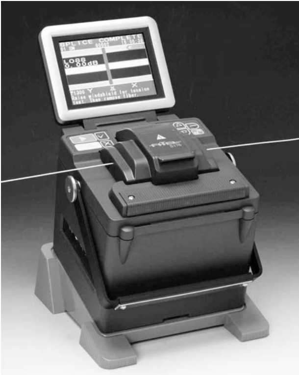
Fig. 10.1. A typical field fusion splicer, the Fitel model S176CR , showing loss estimation following a fusion splice. This unit is compact, lightweight, and can use a battery to facilitate splicing in remote field locations. Like all field splicers, the S176C uses an electric arc as its heat source. The splice includes a profile alignment system (PAS) consisting of a microscope objective, a CCD camera, and a microprocessor. This same system also performs accurate loss estimation. The large LCD screen displays images of the fibers during alignment and following the splice. Simple menu driven software permits the unit to be programmed for a wide variety of fusion splices. A wind screen (deployed over the splice in the image) protects the arc discharge from the ambient environment. The sophisticated capabilities and ergonomic nature of this splicer make it suitable for a factory as well as field environment. Photo courtesy of Furukawa America, Inc.
