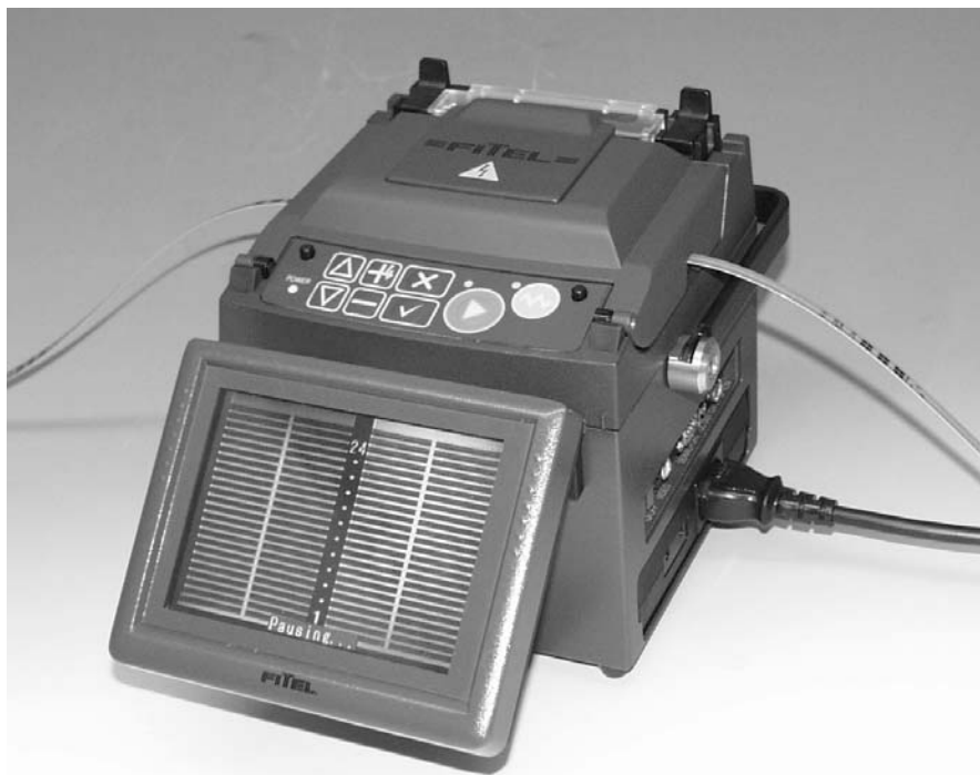
Fig. 10.4. The Fitel S199M24 mass fusion splicer can simultaneously fusion splice all the strands of a 24 fiber ribbon cable. The LCD display on the front of the unit shows two orthogonal views of the 24 individual fiber strands with a small gap between the opposing fiber tips. Typical fusion splice losses are about 0.03 dB for standard single-mode fiber (SMF) and about 0.1 dB for non-zero dispersion-shifted fiber (NZ-DSF). This machine can be used in a field or factory environment. Photo courtesy of Furukawa America, Inc.
