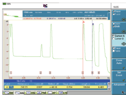
An example of a ghost on the OTDR trace
