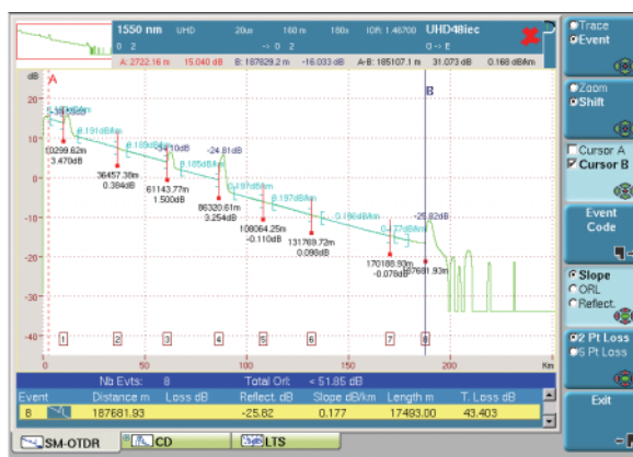
Automatic event detection using the JDSU T-BERD/MTS platforms
