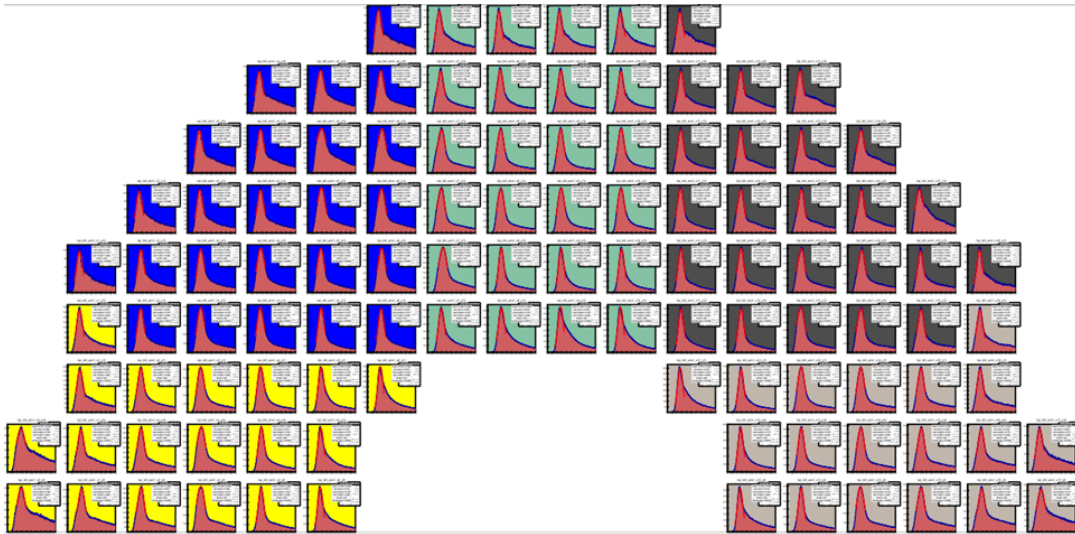
Figure 4.15 The top half of the North MPC. Each plot is a single tower. The color code identifies regions of common electronics. X-axis: Reconstructed mass; Y-axis: Counts.
