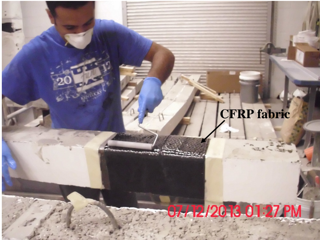
Fig. 4.4 Installation of CFRP fabric at CRP ends.
