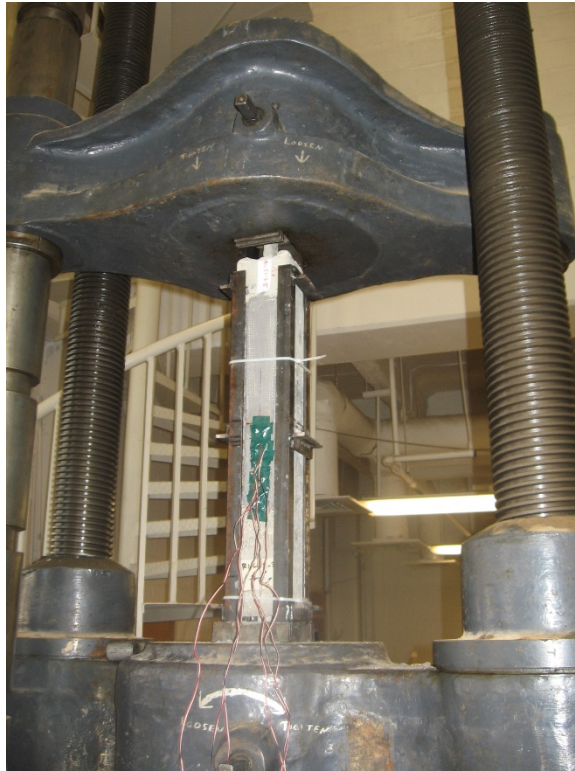
Fig. 3.4 Double-lap shear specimen in testing machine.
