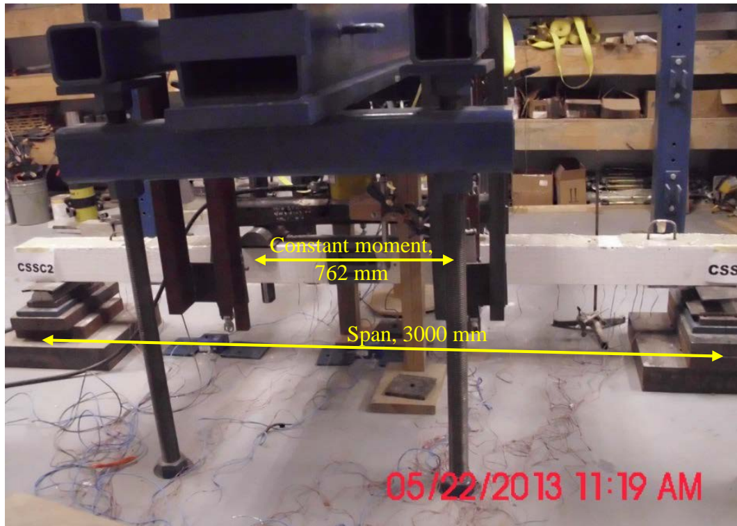
Fig. 4.7 CSSC2 Beam placed in the test frame.
