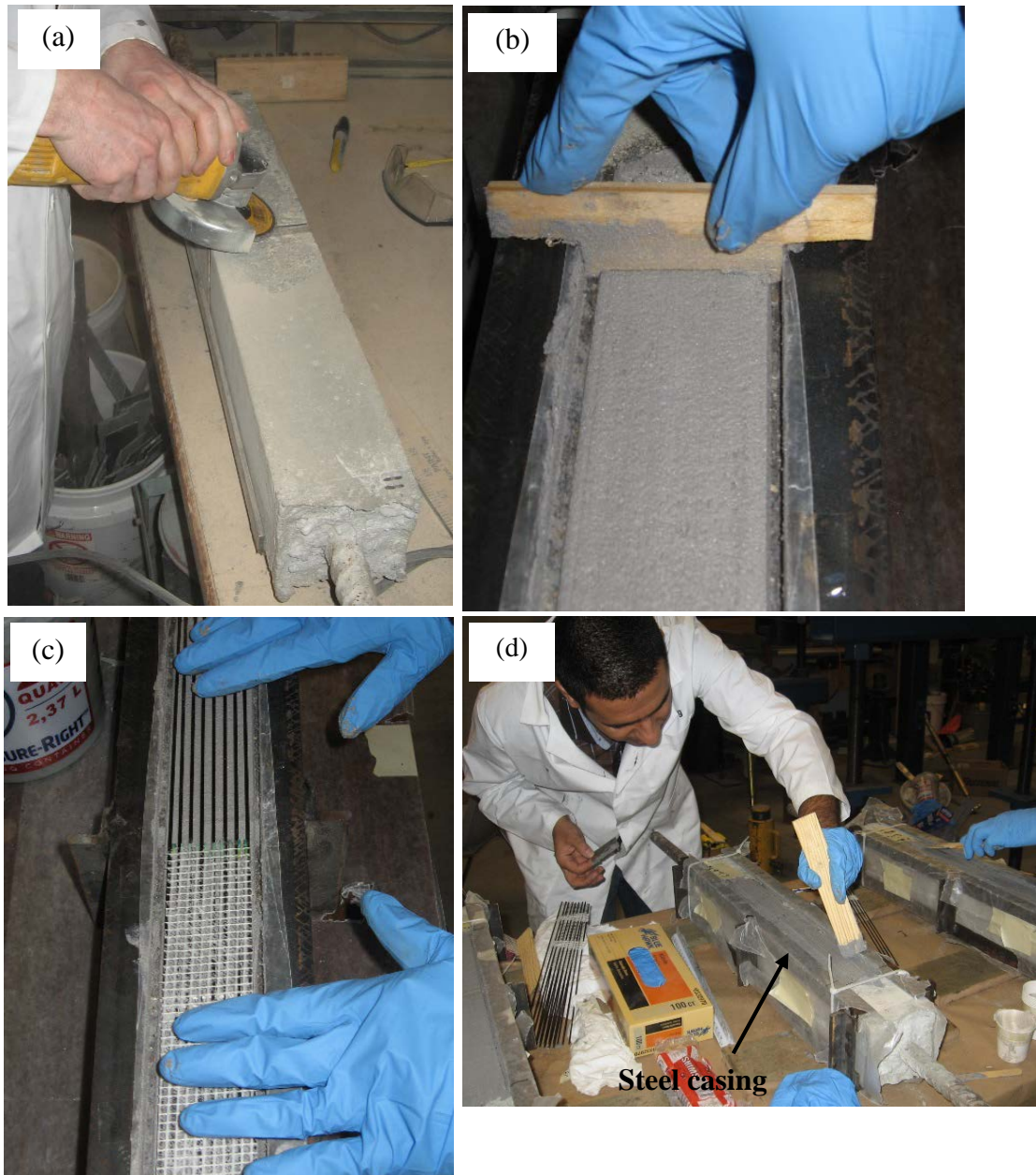
Fig. 3.3 Double lap test specimen fabrication: (a) concrete surface preparation, (b) adhesive application, (c) CRP placement, (d) application of second layer of adhesive.
