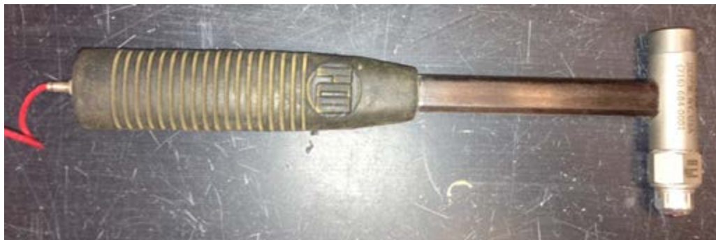
Figure C.37 Electrical Hammer (the exciter) used to generate wave signals
