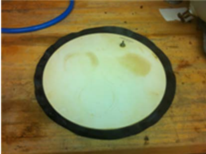
Figure C.2 Typical pressure plate used in the SWCC pressure chamber, (a high air-entry porous ceramic disk with rubber ring).
