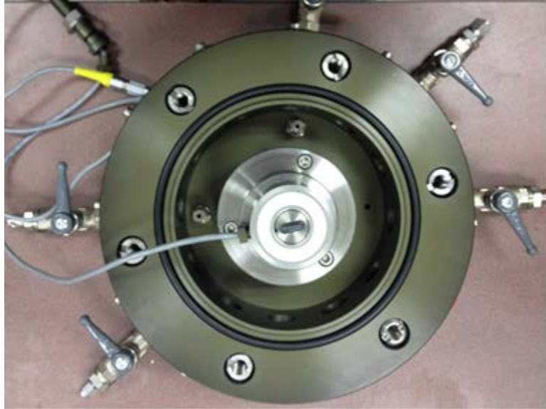
Figure C.24 Base pedestal of double walled unsaturated triaxial cell showing HAEPD and bender element centered on base pedestal.
