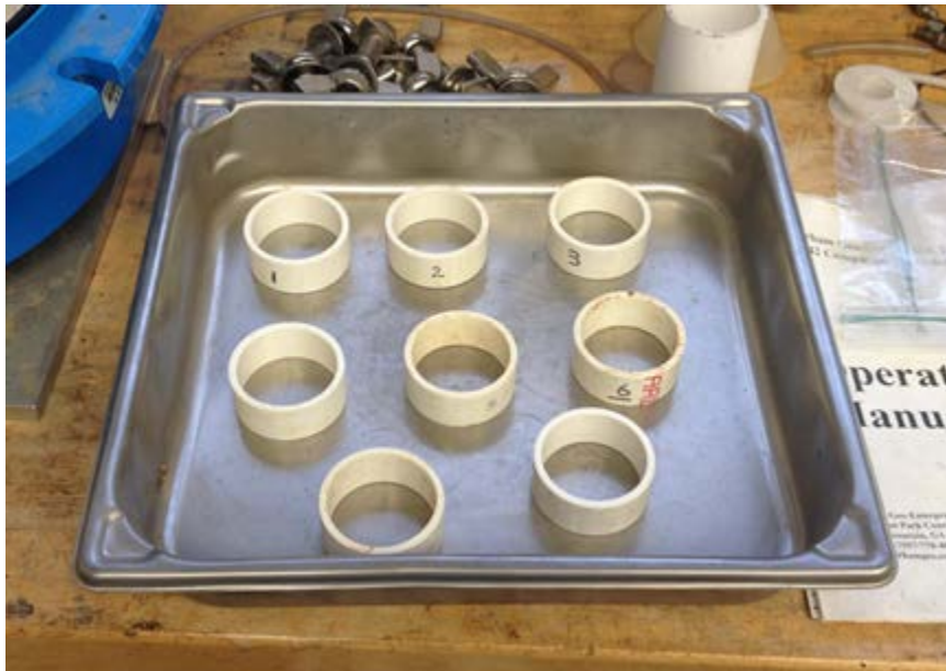
Figure C.5 Retaining rings for soil-water retention tests machined cut from a Schedule 40, PVC pipe.
