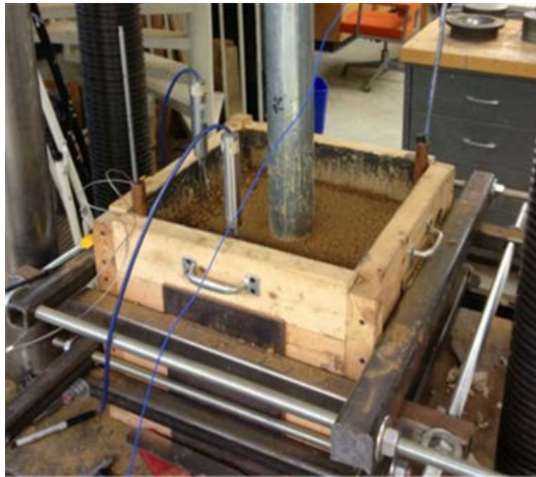
Figure C.40 Shelby tube sampling of the bulk soil.
