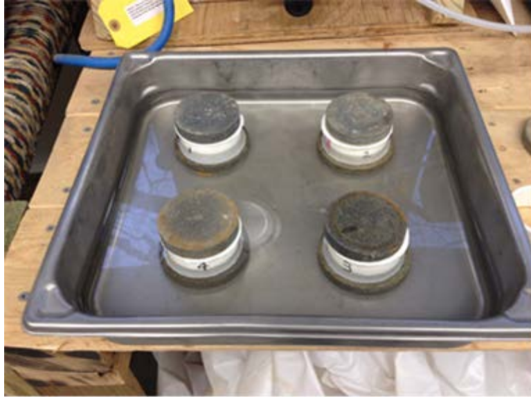
Figure C.11 De-aired water poured around SWCC samples sandwiched between porous stones and filter paper, to a depth below the top of the specimens.
