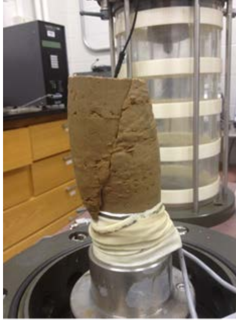
Figure 7.26 Slip plane failure, and offset from horizontal of the top of specimen S-CW-DC-16.4-1730.
