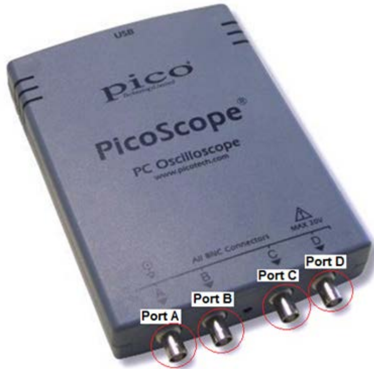
Figure C.36 Photo of the PicoScope oscillator, Model 3200.
