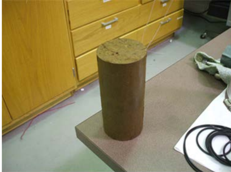
Figure C.19 Typical CIU triaxial soil specimen.
