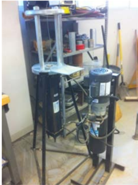
Figure C.6 Static Compactor and Extruder
