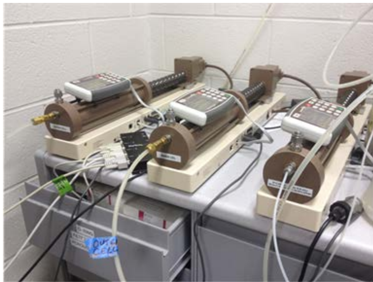
Figure C.23 Standard pressure volume controller v2, STDDPC.
