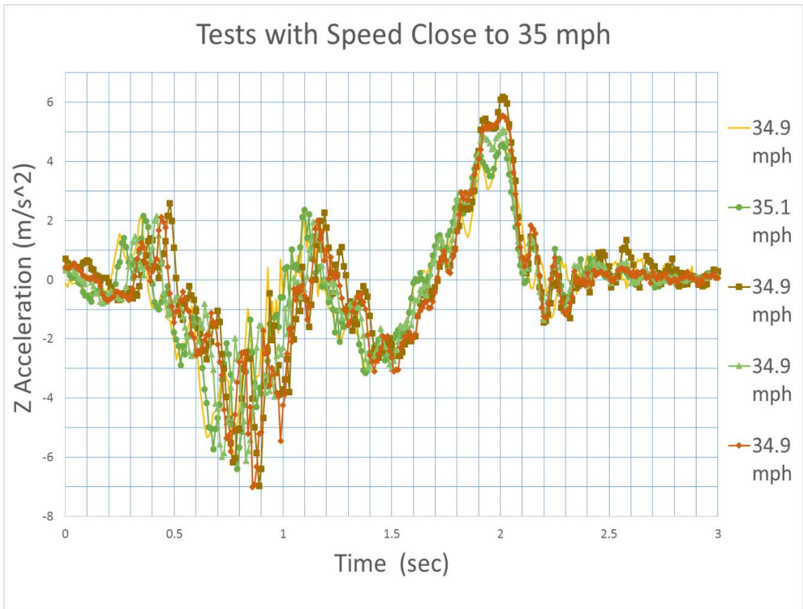
Figure 5.2 Accelerations measured at speeds close to 35 mph.
