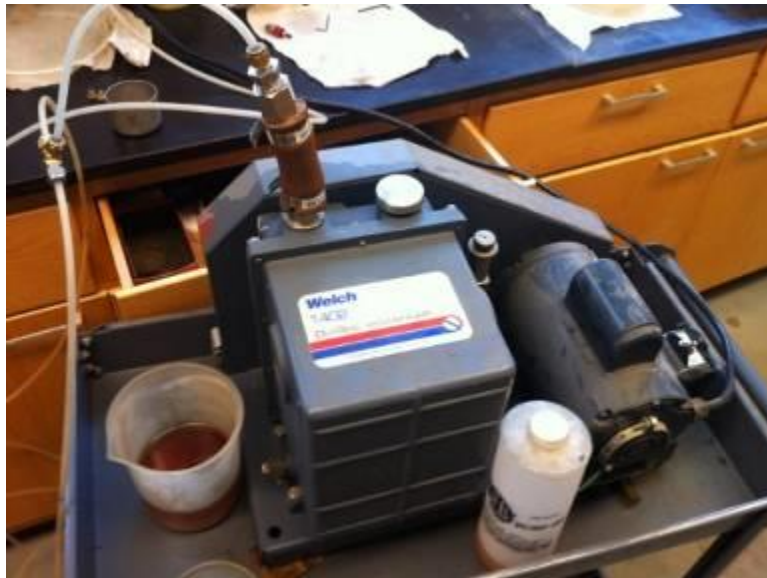
Figure B.14: Welch Dual Seal Vacuum pump
