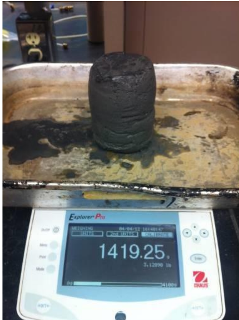
Figure B.17: Measuring the specimen weight after testing
