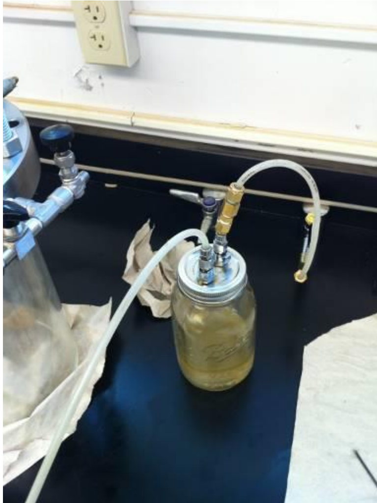
Figure B.6: Vacuum water trap
