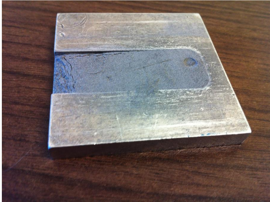
Figure 4.3: Sample holder for the X-Ray diffraction (XRD) test
