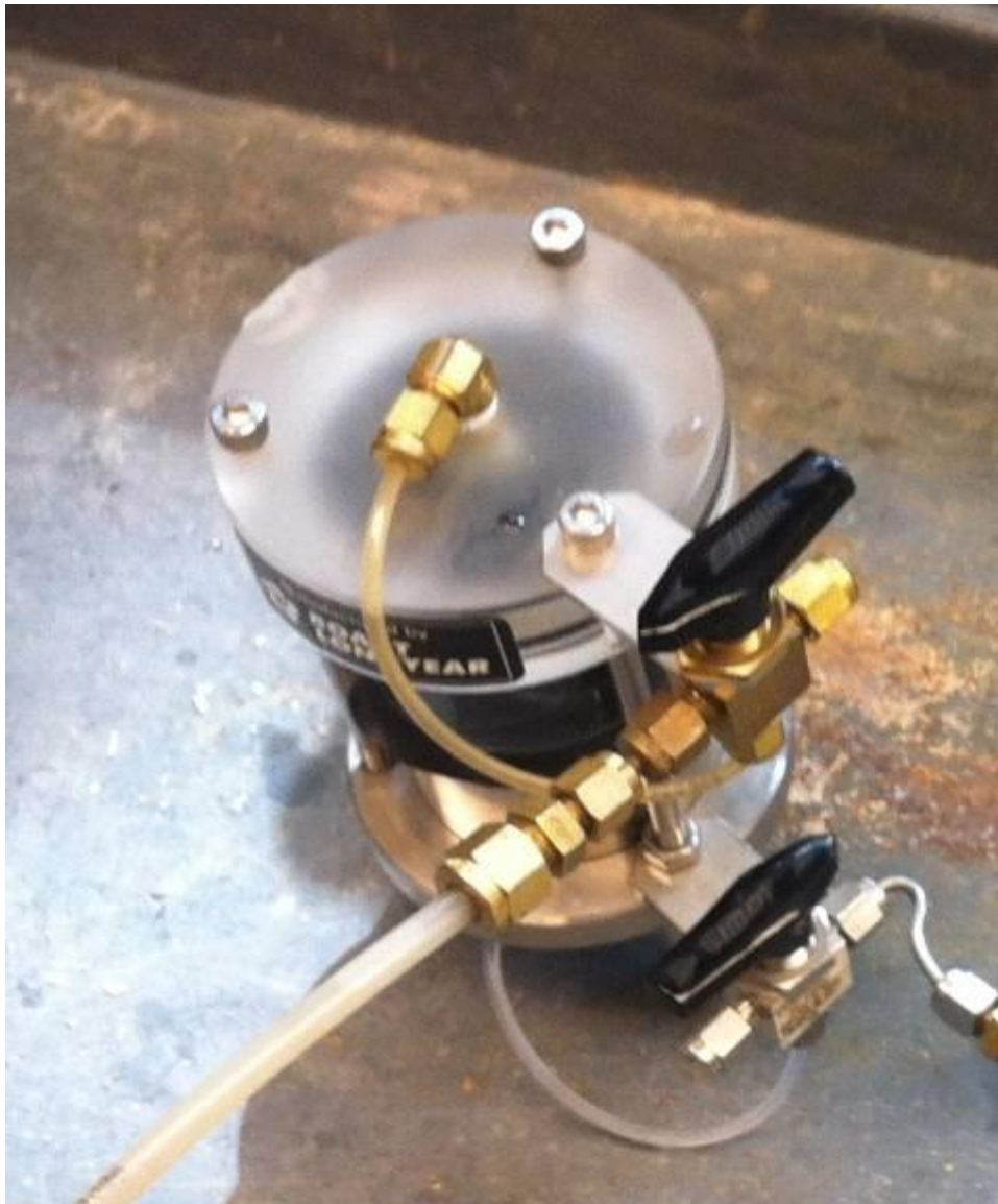
Figure B.16: Contamination separation chamber
