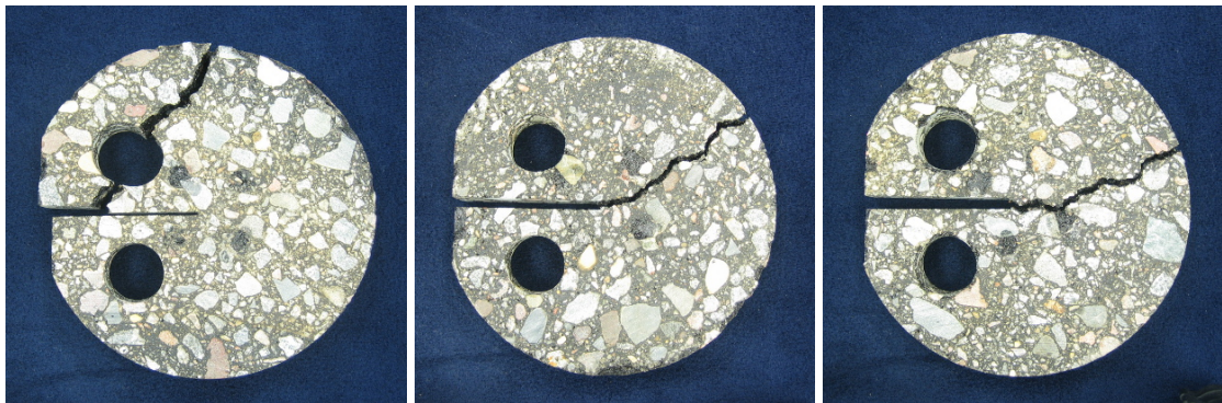
Figure 1.4. Imperfections in the Failure of DC(t) Specimens
