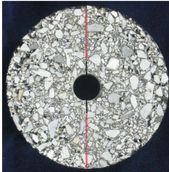
Figure 3.6. Fabricated IRT Specimen
