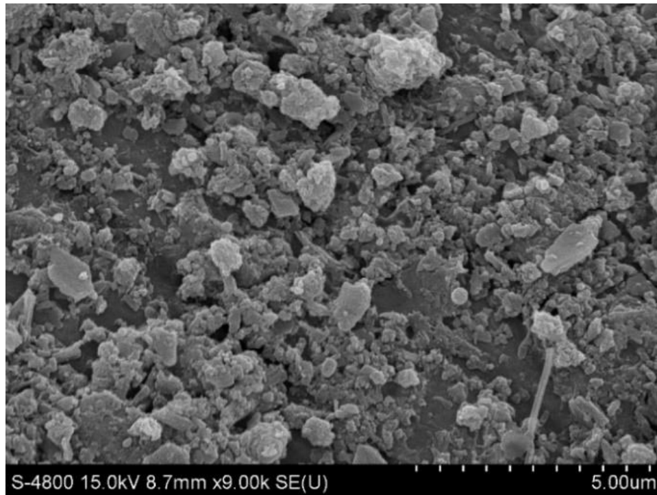
Figure 5-3. SEM image of OPC paste showing irregular structure of C-S-H phases; 9000x magnification.
