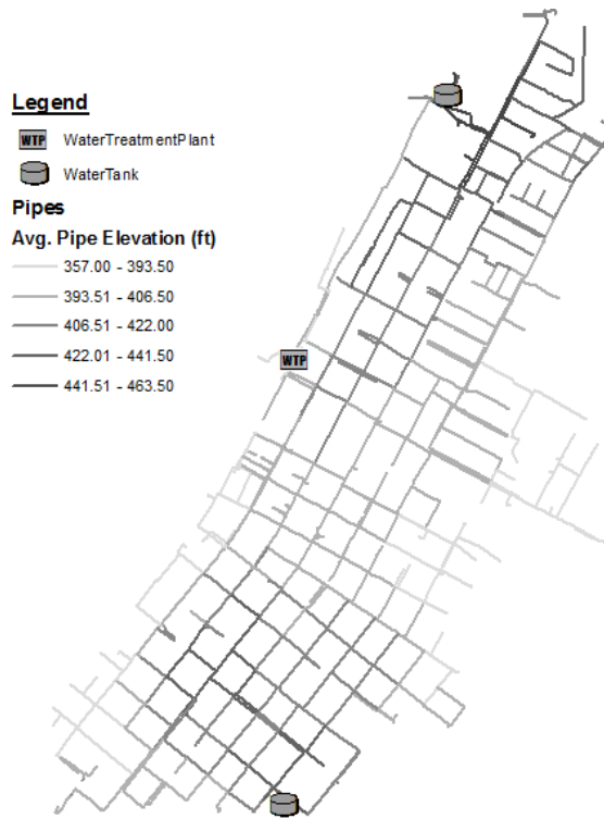
Figure C.7: Average Pipe Elevation for KY1.
