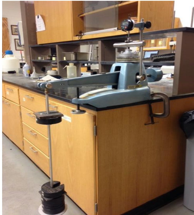
Figure 6.2 Consolidation load frame
