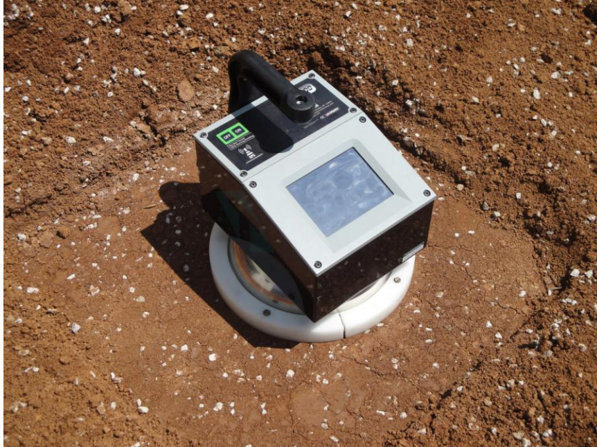
Figure 2.3: Soil Density Gauge 200 developed by TransTech Systems Inc.
