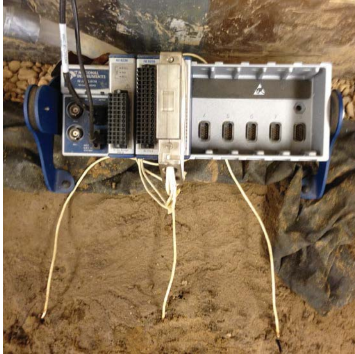
Figure 3.3: Three pore pressure transducers connected to the National Instruments data acquisition system.
