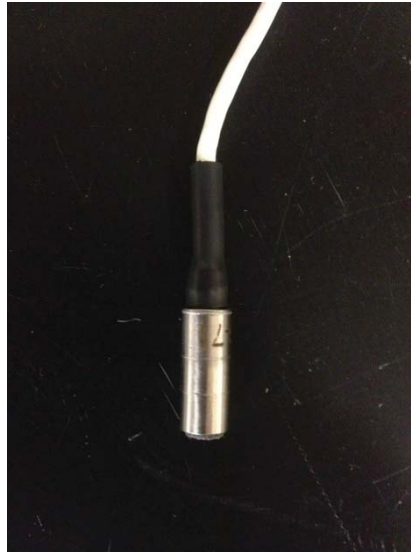
Figure 3.4: Kulite's XCL-11-250-150SG sealed gauge pore pressure transducer model used in this study.
