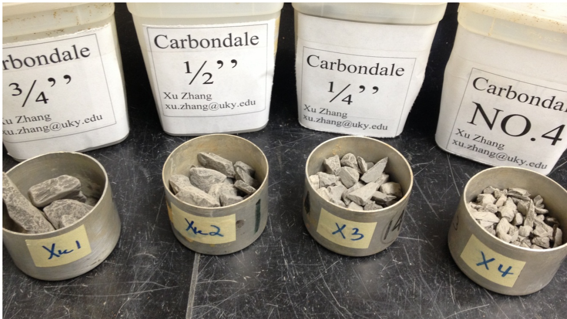
Figure A-23 Demonstration of Specimen Size of Electrical Jar Test
