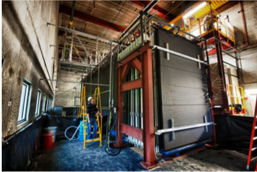
Figure 1.7: The fully constructed NDOS at Fermilab in the surface building. This shows the NDOS from the muon catcher (back) end of the detector. A physicist stands beside the detector during commissioning and shows the relative size of the detector.
