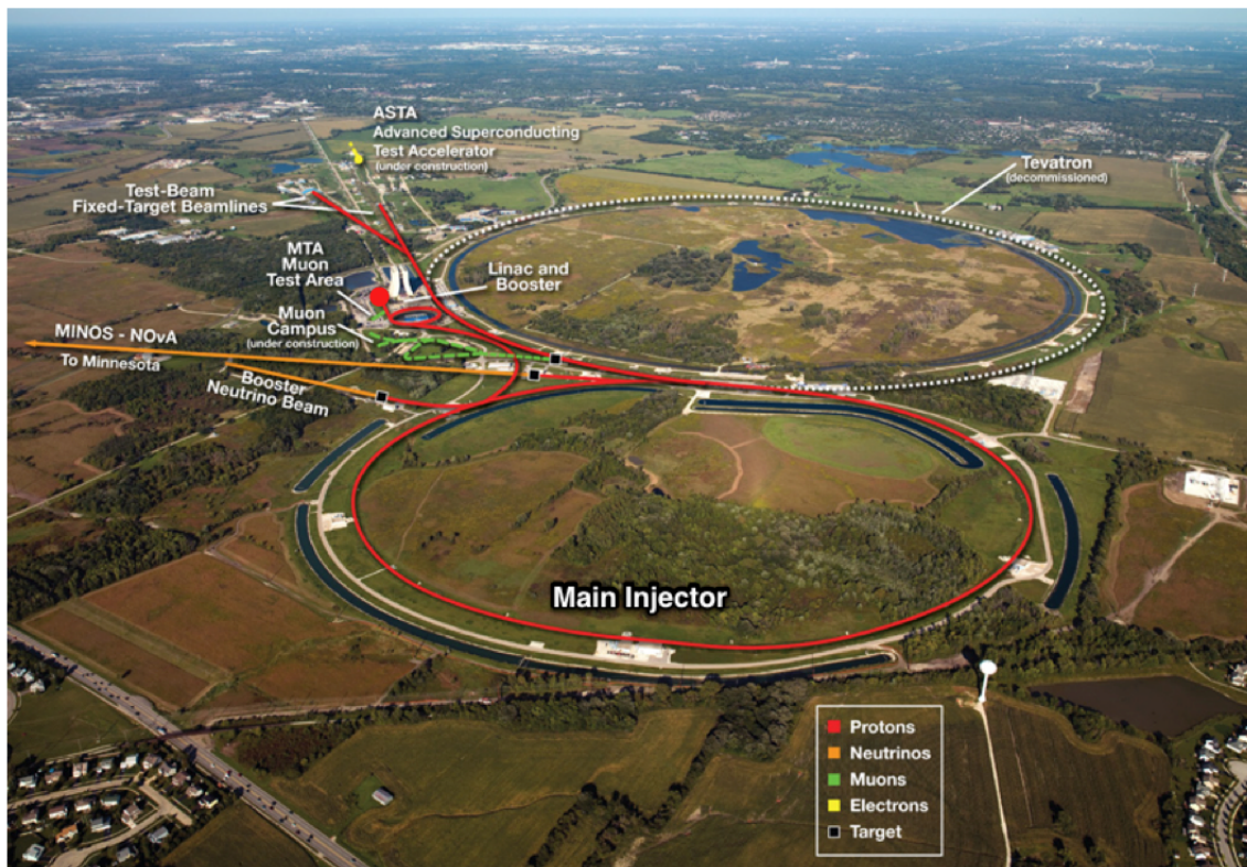
Figure 1.1: An aerial photograph of the accelerating rings and neutrino beams at Fermilab. Courtesy of Fermi National Accelerator Laboratory.
