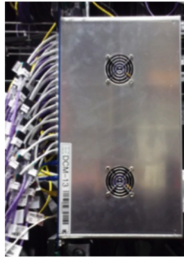
Figure 1.12: A photograph of a DCM where up to 64 FEBs synchronize data collected in a spill window to then be stored in a computer for later processing.
