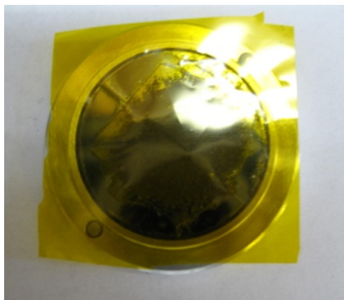
Figure 3.7 Air-sensitive sample for powder X-ray diffraction sealed by Kapton film.
