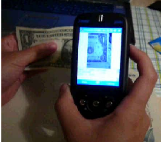
Figure 5.8: Currency reader for the visually impaired
