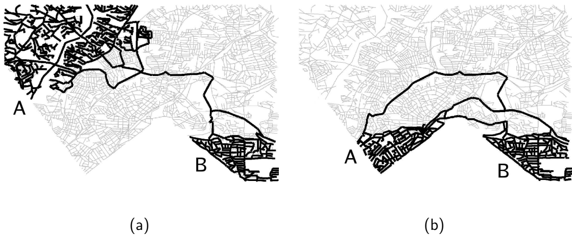
Figure 5.1: Two subsets A, B of vertices in a road network of Silver Spring, MD. The shortest paths between all pairs of vertices in A and B are marked in a darker shade. (a) The 30,000 shortest paths pass through a single vertex, and (b) the 20,000 shortest paths that pass through one of the two vertices
