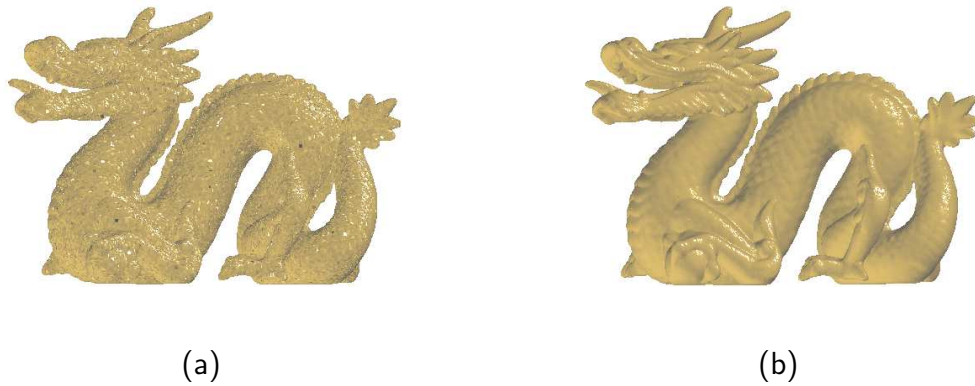
Figure 7.16: (a) A noisy mesh-model of a dragon, and (b) the corresponding model whose surface normals were recomputed using our kNN algorithm. The algorithm took about 118 seconds and used 8 neighbors.
