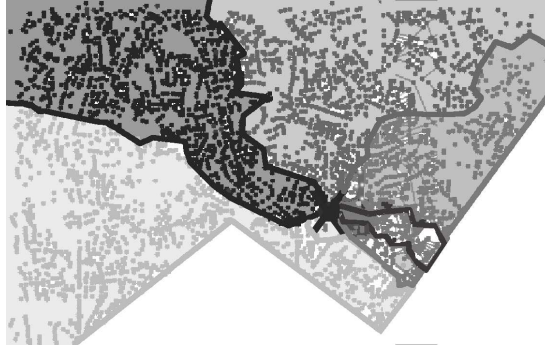
Figure 2.1: Partition of the underlying space spanned by the spatial network in Figure 1.1 into regions r_i such that the shortest path from the vertex marked by X to a vertex in r_i passes through the same vertex among the six vertices that are adjacent to X (i.e., the shortest-path map of X).
