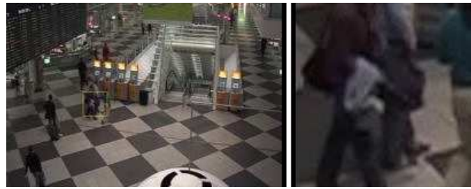
Figure 2.3: Using window energy density as a measure of motion energy favors smaller windows, cropping away small parts of objects, such as heads in humans (left: original frame, showing the location of the cropping window; right: cropped frame).
