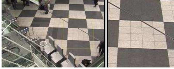
Figure 2.15: A cropped frame resulting from panning across a largely empty scene (left: original frame, showing the location of the cropping window; right: cropped frame).
