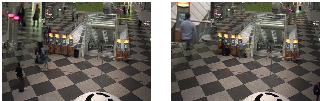
Figure 2.10: Video-in-video results: the cropped video location is selected automatically in the boundary region of overall least activity.
