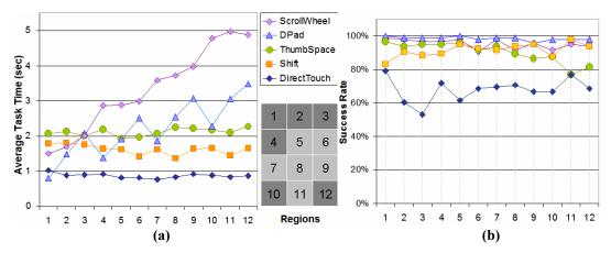
Figure 41. ThumbSpace Study 1: Average task times (a) and success rates (b) by region for each input type.
