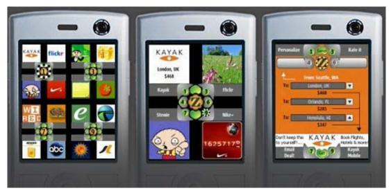
Figure 26. The three zoom levels of Zumobi, a commercialization of the LaunchTile design.
