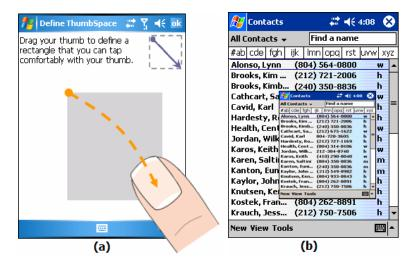
Figure 34. An example of how users define a ThumbSpace (a), and an example of a ThumbSpace depicted as a Radar View (b).
