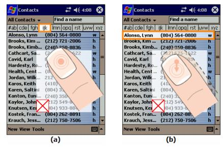
Figure 36. An example of how a user selects an object using ThumbSpace. Assuming the user wants to select the first name in the Contacts list, she first aims at the ThumbSpace proxy for 'Alonso' (a). Since the user's initial ThumbSpace contact point maps to 'ijk', she adjusts the selection by dragging her thumb toward the bottom of the screen (b). The user confirms the selection by lifting her thumb.
