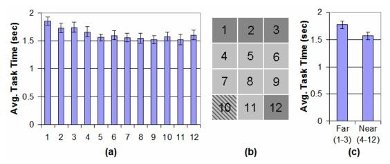
Figure 44. ThumbSpace Study 2: Average task times by input region. Average task times by region (a). User-defined "hard to reach" (dark) and "easy to reach" (light) regions (b). Average task time by distances "far" and "near" (c). Regions (1-3) were considered "far" because the majority of users thought those regions were hard to reach, and distance is the most reasonable explanation for why they thought this. All other regions, by contrast, were considered "near".
