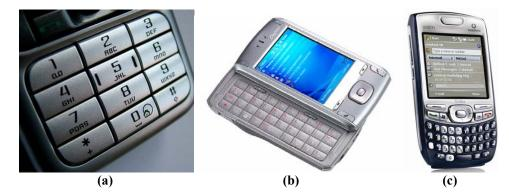
Figure 2. Examples of mobile device keyboards. The assignment of letters to buttons for a standard phone keypad (a). A cell phone model with a slide-out Qwerty thumbboard (b). A phone model with an integrated thumbboard on the front of the device (c).
