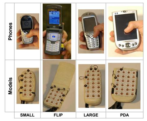
Figure 9. Thumb Movement Study: Devices used for the thumb movement study, chosen to represent a range of sizes and forms (top row), together with their study-ready models (bottom row).
