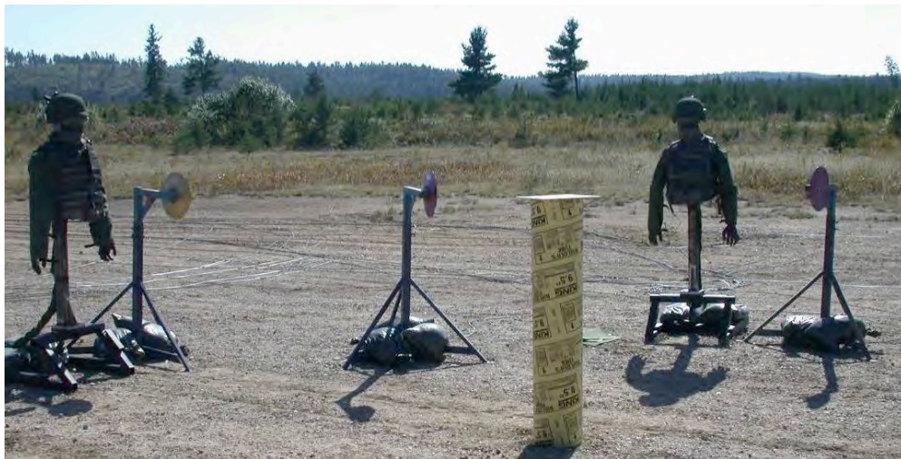
Figure 1.2: Photograph of experimental set-up with two mannequins facing forward, toward the blast. Center pillar was a high explosive, which generated the blast wave once
