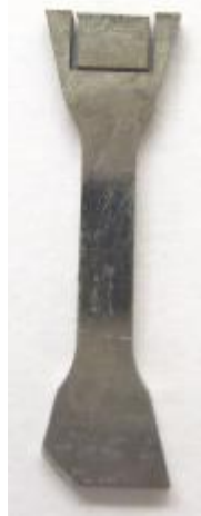
Figure 4.40: Photo of a dogbone with the rectangular indentation sample cut using wire electrical discharge machining.
