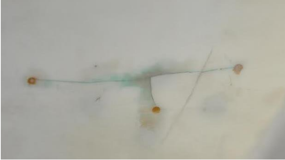
Figure 22: MACOR crack repair
