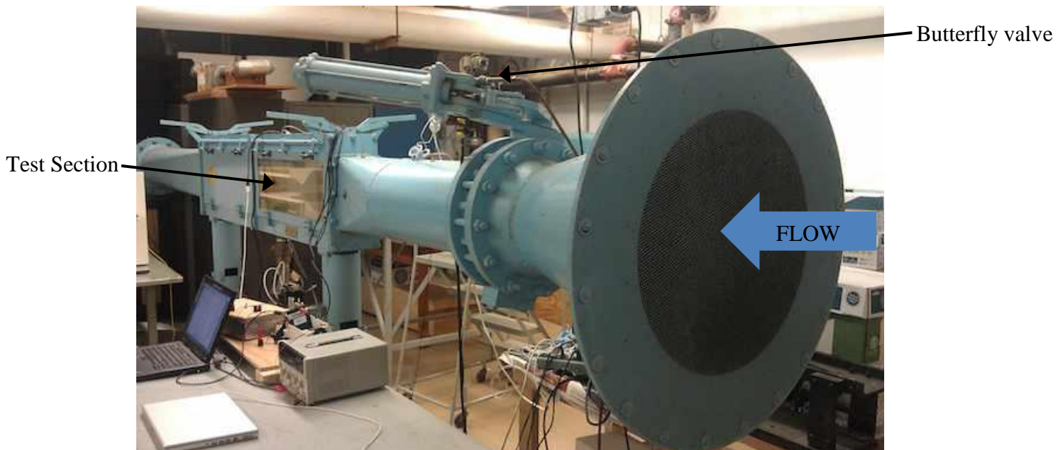
Figure 4: University of Maryland supersonic wind tunnel
