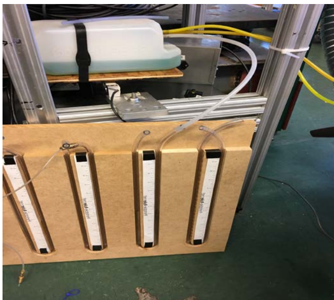
Figure 3.7: Hand-made water manometer to gas tank
