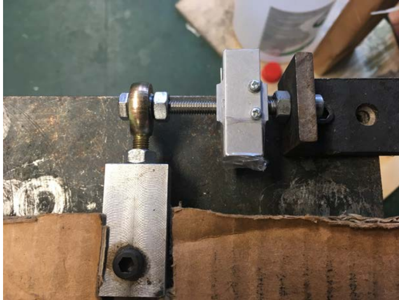
Figure 3.2: Close up view on load cell
