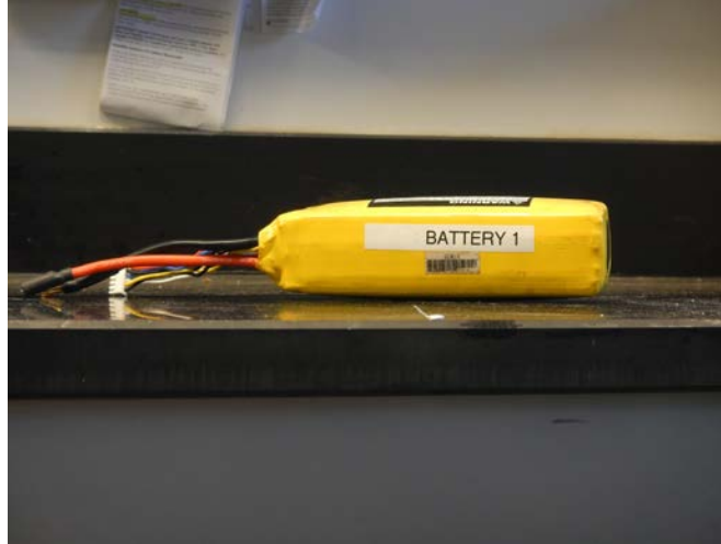
Figure 3.14: Zippy Compact LiPo battery swollen
