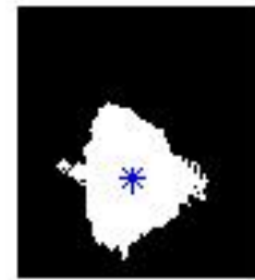
Figure 4-2. Reflection from the top electrode and associated centroid location.
