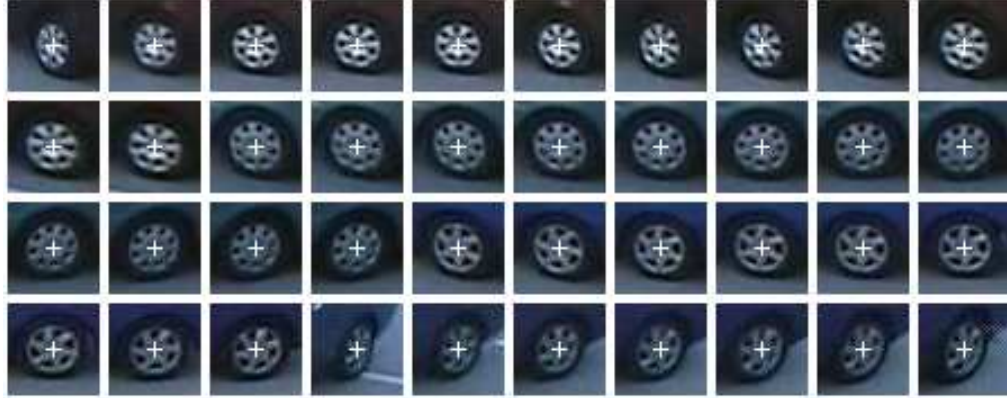
Figure 7.10: Sample of detected wheels. The detected wheel centers are indicated by white crosses
