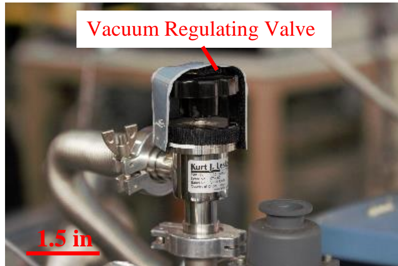
FIGURE 12 – Diagram depicts the regulating valve on the vacuum pump used in conjunction with the mass flow meter to control the pressure of the plasma cell.
