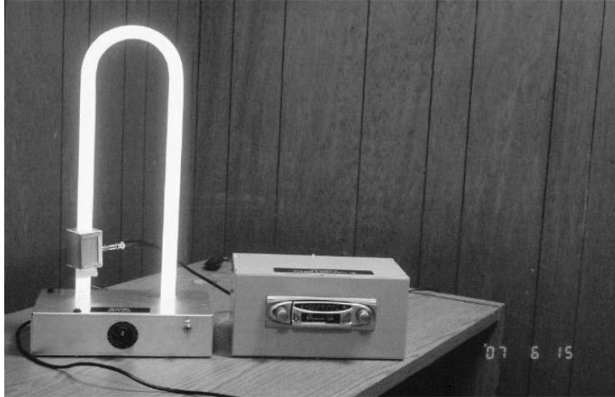
FIGURE 2 – Picture of a plasma antenna made from a neon tube [4].
