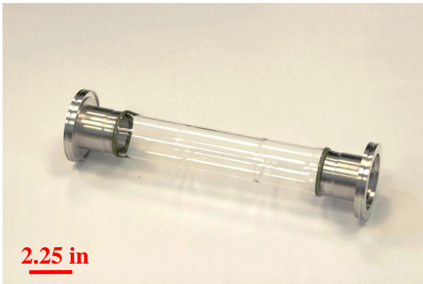
FIGURE 8 – Picture of the ISO-63K glass tube design employed in the final plasma experiment.
