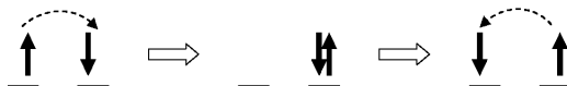
Figure 2.2 Illustration of the virtual exchange process between two electrons of opposite spins on the nearby sites. Each arrow denotes an electron of specific spin. The initial occupation is shown to the left of the figure. As the spin up electron hops to the right site, an intermediate configuration is produced having an empty and a doubly occupied site next to each other. Then, very rapidly, the spin down electron hops back to the left site and the final configuration is shown on the right of the figure. Through this process, the system develops an exchange energy of J = 2t^2/U .
