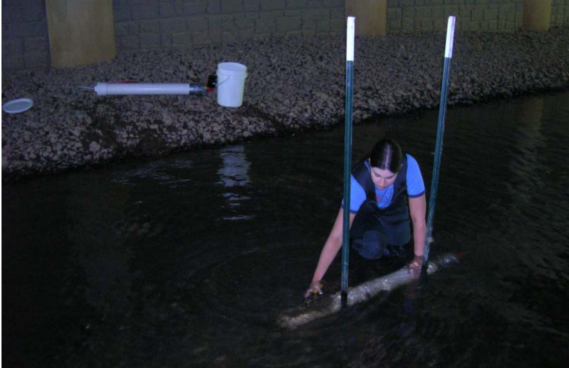
Figure 4-3) In-situ sediment trap implemented in the field
