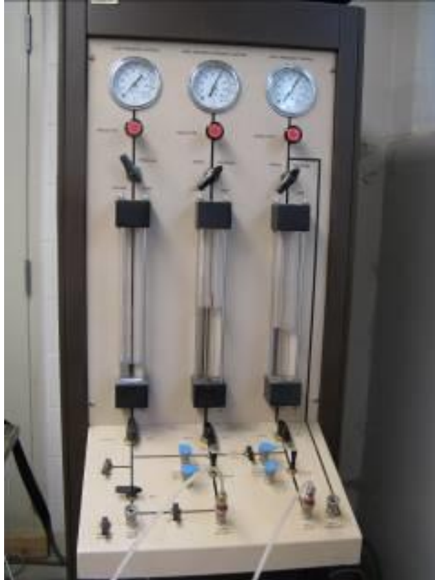
Figure B.4: Pressure board containing the burettes, regulators, and the valves.
