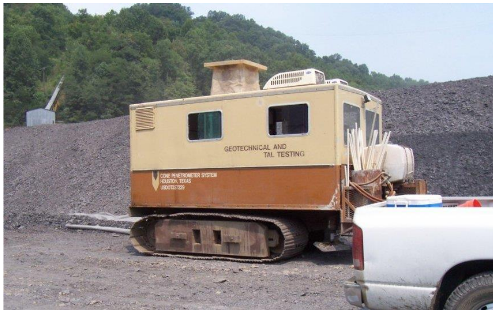
Figure 2.8: CPT equipment used at the Big Branch impoundment.
