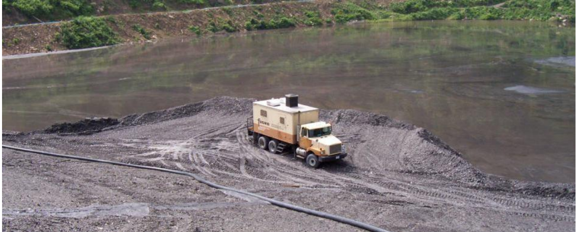
Figure 2.7: Performing sCPTu test at location B (beach, toe) at Abner Fork.
