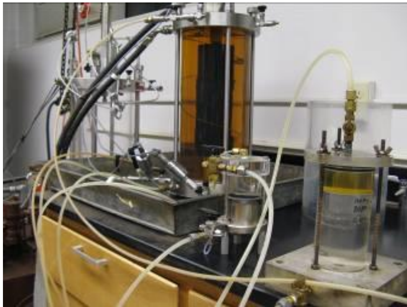
Figure B.15: The chamber filled with oil and the intermediate cell to transfer pressure from water to oil.
