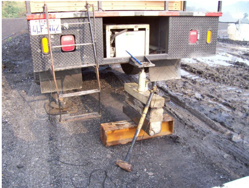
Figure 2.10: Performing seismic CPT test using a sledge hammer.
