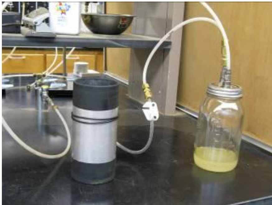
Figure B.12: Stretching the membrane by applying vacuum.
