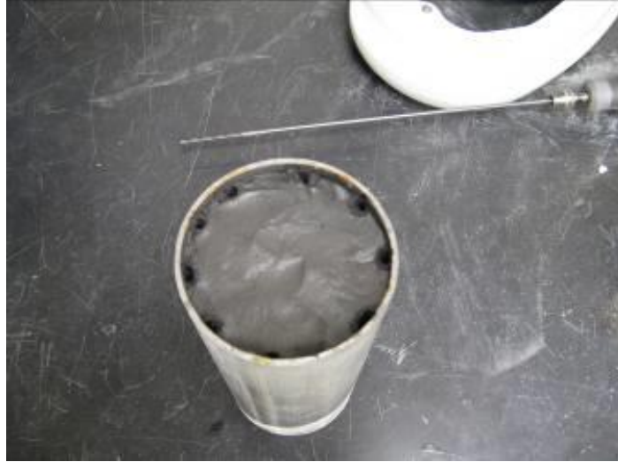
Figure B.8: Drilled holes to relieve negative pressure during sample extruding.
