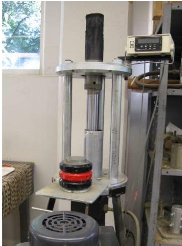
Figure B.9: The hydraulic jack for extruding the specimen.
