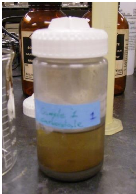
Figure A7. Reaction to iron oxides removal procedure for the carbondale shale.
