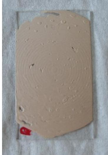
Figure A15. Slide with sample after pretreatment used to run the XRD test.
