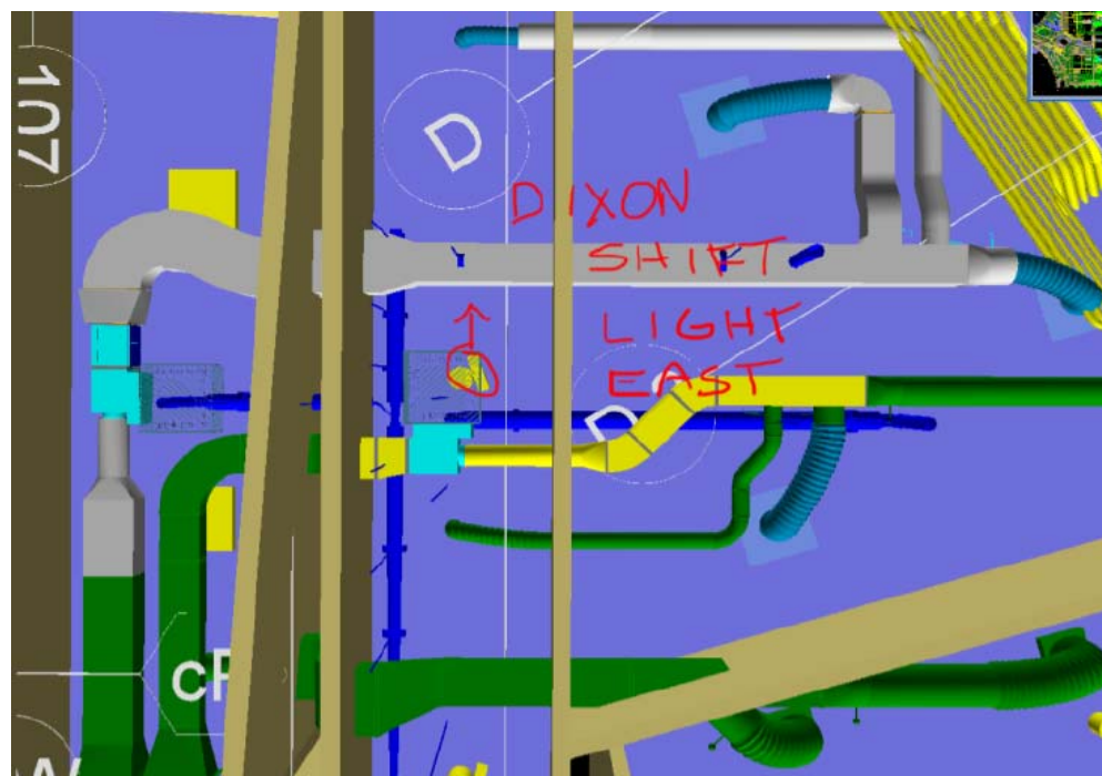
Figure 7.22: Example 9 – Shift Light to Avoid Access Door
