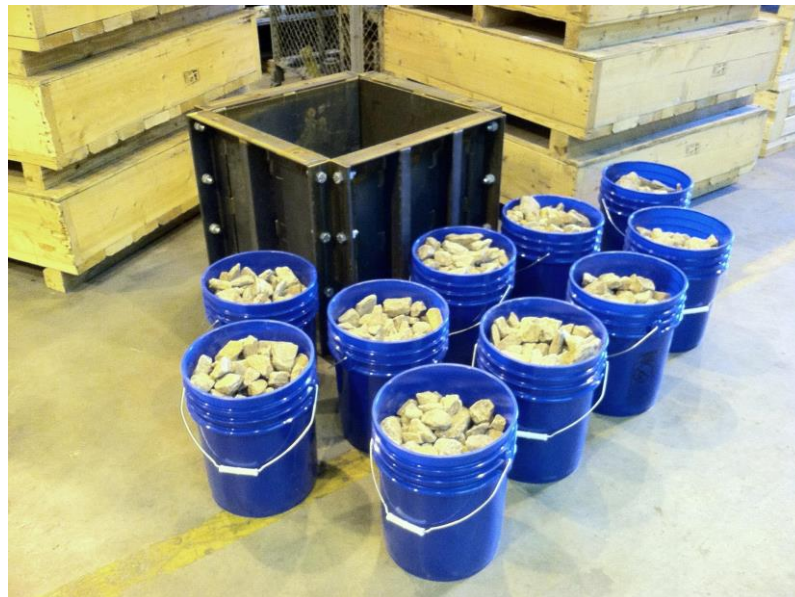
Figure 5.2 Steel ballast box and nine five-gallon buckets of ballast
