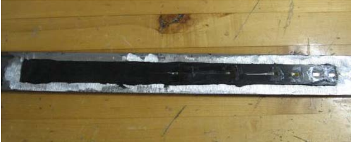
Fig. 2.25: Doubly Reinforced Steel Plate with attached Strain Gages
