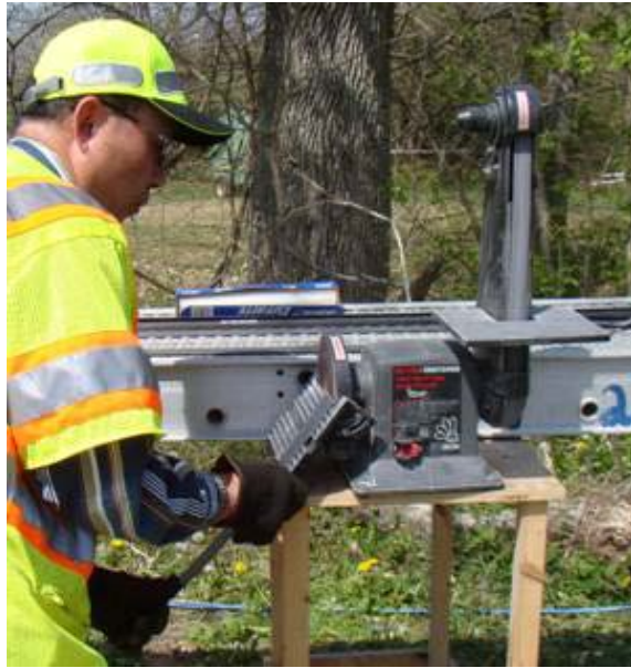
Fig. 5.16: Sanding laminate edges to obtain reverse taper
