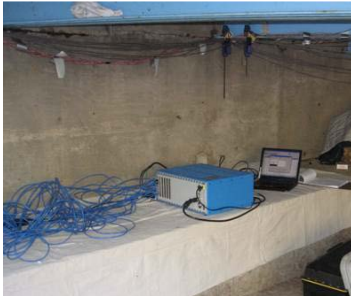
Fig. 5.30: Separate data acquisition system and laptop for laminate strain data
