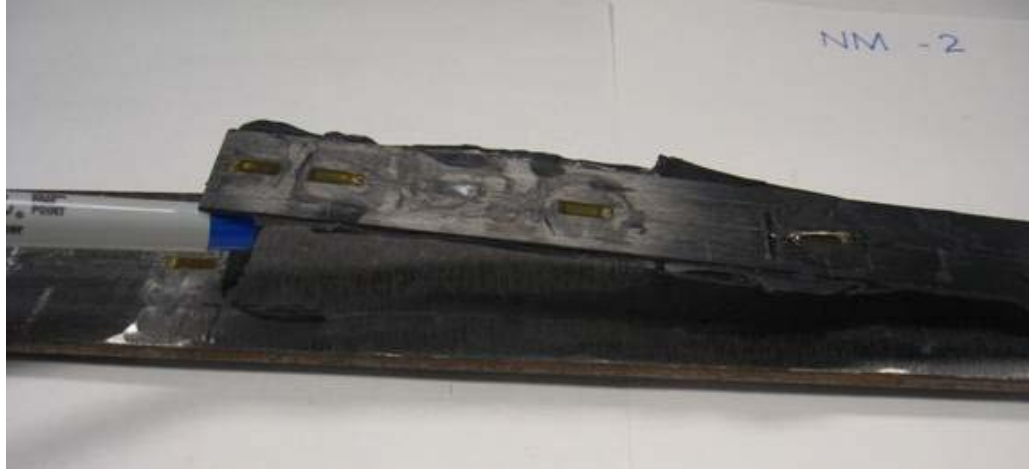
Fig. 2.28: Debonding observed in doubly reinforced steel specimens
