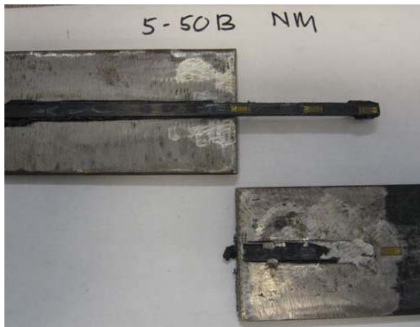
Fig. 2.11: Typical combined steel-epoxy interface debonding and CFRP delamination seen in normal modulus CFRP
