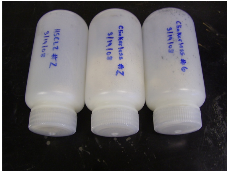
Figure 5.1 – Photograph of sealed plastic containers with moist paper towels stored at room temperature used in the refined method of curing the cement paste samples.
