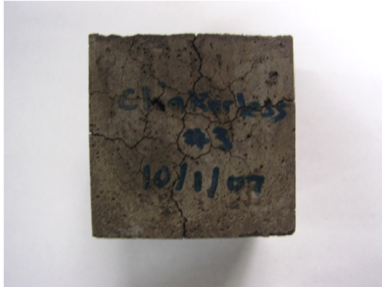
Figure 6.3 – Photograph of map cracking on a mortar cube prepared using the Clinkerless #3 cement blend after 56 days in the moist curing room.
