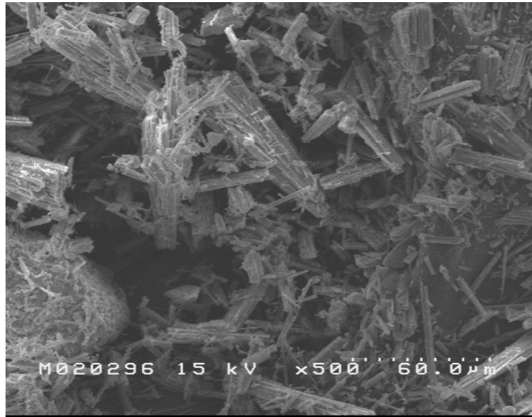
Figure 6.24 – SEM photograph of hemihydrate crystals produced from gypsum that was pressed into pucks with 48.93 kN (11000 lbs) of force, and autoclaved four hours.
