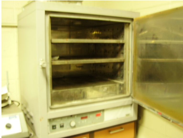
Figure 4.6 – Photograph of the VWR Scientific Model 1370 FM Forced Air Oven used for the drying phase of the hemihydrate processing.
