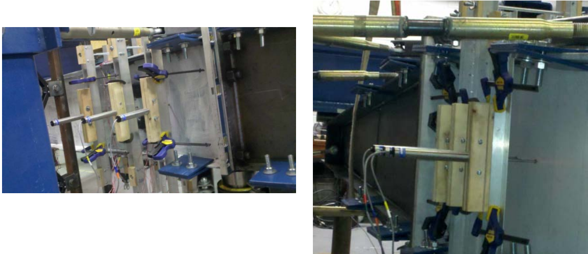
Figure 2-8 LVDTs for Web Out-of-Plane Measurements
