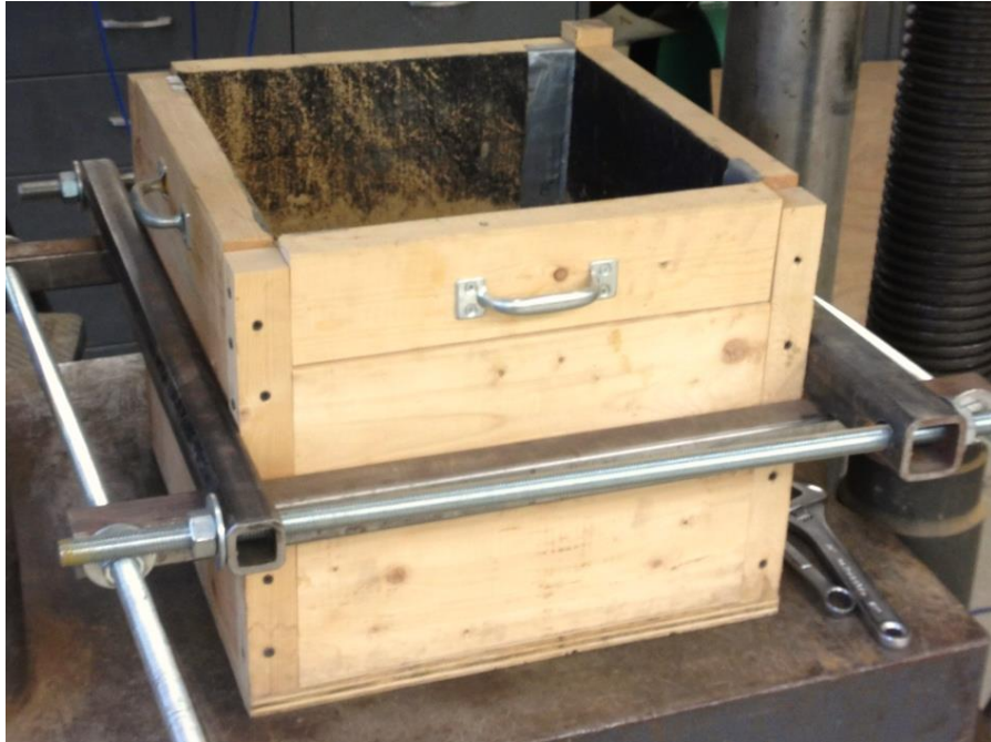
Figure 3.11: Testing box with bracing
