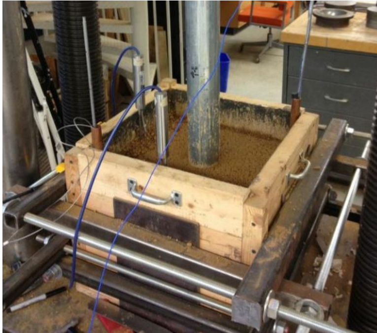
Figure 3.15: A shelly tube being driven into the compressed soil by the load frame
