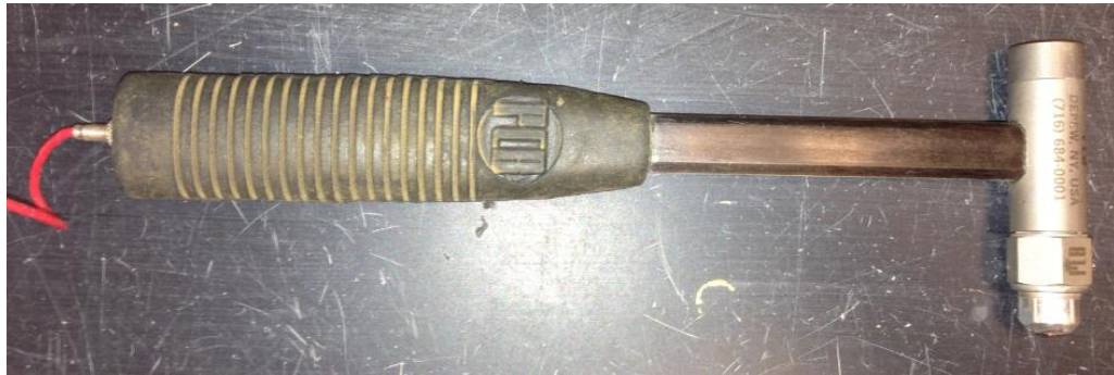
Figure 3.4: Hammer used to create the source of the shear waves
