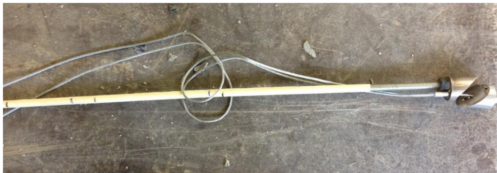
Figure 3.5: Rod with a wedge used send shear waves at a controlled depth
